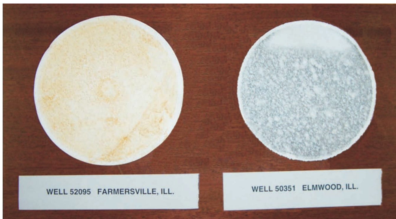
Figure 6. Examples of clay-sized particulates on filter media for samples collected from two public-supply wells that tap source-water aquifers in Illinois, 2001-02 (filter diameter is 142 millimeters—about 5.5 inches; refer to figure 3, Montgomery Co. and Peoria Co., respectively, for well locations).
