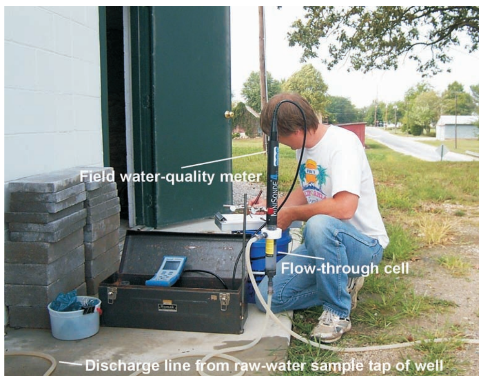
Figure 4. Monitoring of field water-quality characteristics (temperature, pH, specific conductance, oxidation-reduction potential) for stabilization of values prior to collection of ground-water samples.
