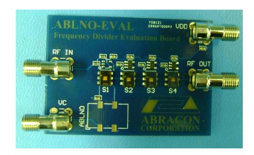
Abracon also offers an Evaluation Board to assist engineers & technicians with quick evaluation of the ABLNO oscillators. This evaluation board can also be used to characterize reference clocks, other than the ABLNO. Please download a comprehensive data sheet by visiting this link: <a href="http://www.abracon.com/Precisiontiming/ABLNO-EVAL.pdf">http://www.abracon.com/Precisiontiming/ABLNO-EVAL.pdf</a>
