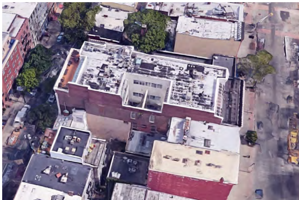
Figure 16. Google Earth view of Geismar-Meyer Co. Department Store building showing the penthouse level addition and the lightwell inserted on the south side of the structure (Source: Google).
