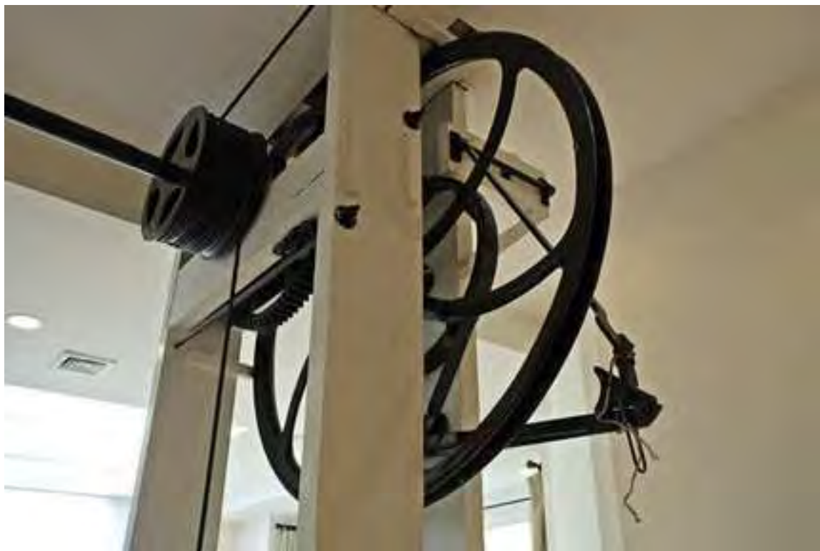
Photograph 4. Image of the reportedly 100-year old elevator system, from 2010 listing (Maurer 2010).
