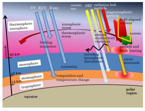
Figure 39. Impact of the sun on the Earth's ionosphere and atmosphere. The figure is cited and partly modified from "Present and Future of the Society of Geomagnetism and Earth, Planetary and Space Sciences" (SGEPSS, January 2013).
