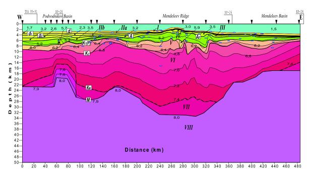
Figure 48: Seismic velocity structure near the Mendeleev Ridge (Lebedeva-Ivanova, et al., 2006)
