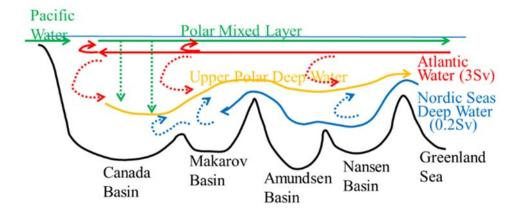
Figure 18: Ocean circulation in the Arctic Ocean on the vertical cross-section from the Bering Strait to the Fram Strait. The total ocean depth is about 4000m, and the Atlantic Water flow in red occupies the depth of 300~700m. The solid lines denote clear currents, and the dotted lines denote mixture of weak currents and mixing. The dotted lines have not been clarified well yet.
