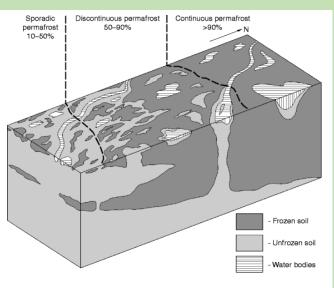
Figure 53: Schematic diagram of three-dimensional distribution of permafrost and the classification of continuous, discontinuous, and sporadic permafrost (Encyclopedia of Snow, Ice and Glaciers).
