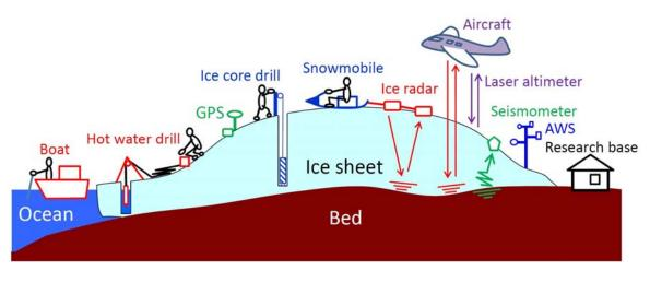
Figure 69: Field equipment and facilities for glacier and ice sheet research.
