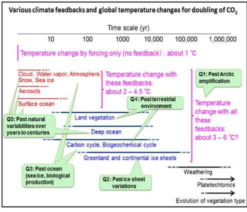
Figure 21: Climate feedbacks and resulting global temperature changes under doubling  $CO_2$ . The timescales of each climate component, as well as the relationship between the questions in the text and climate components, are also shown. [Theme 6]
