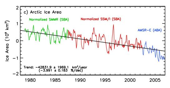
Figure 57: Changes in deviations in the northern hemisphere sea ice area, as observed by microwave radiometer (from Comiso and Nishio, 2008).
