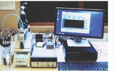
The Scripps total alkalinity titration system has been designed and optimized for accurate measurement of the total alkalinity of discrete seawater samples. It is essentially identical to the system currently used in the Scripps CO<sub>2</sub> Reference Material Program to assign total alkalinity values to our CO<sub>2</sub> in seawater reference materials. The same design of system is also used for at-sea measurements of total alkalinity made during the US Repeat Hydrography Program.
