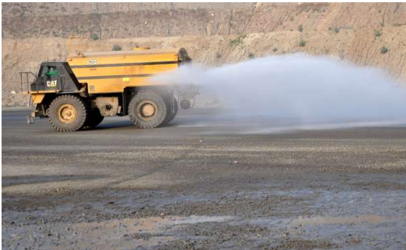
40KL Water sprinkler
