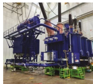
Figure 1 | Synthetic ester oil transformer - 400kV 240MVA
