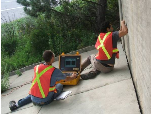
Figure 7.12. Non-destructive testing of ASR-affected concrete structures. A. Impact-echo. B. Non-linear acoustic technique.
