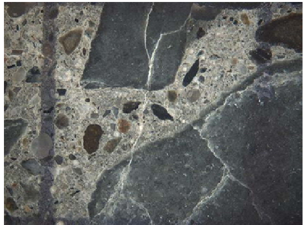
Figure 7.14. A. Highway bridge affected by ASR in Bangor, Maine. Coring sites in the abutment (not exposed (site 1 - B) and the wing wall (exposed (site 3 - C)). D. DRI results for cores obtained from sites 1 to 3; the higher the DRI, the higher the degree of ASR damage in the concrete. E. Polished section from site 1 showing very limited signs of deterioration. F. Polished section from site 3 showing extensive cracking filled with alkali-silica gel in aggregate particles and the cement paste.
