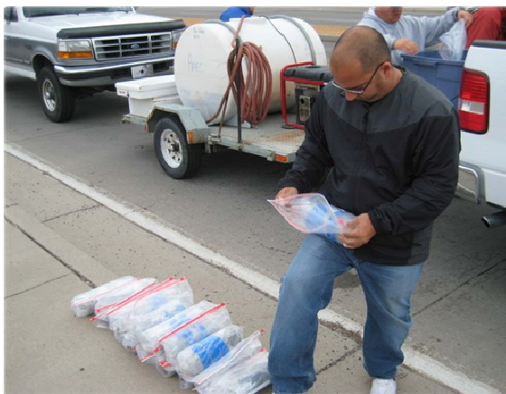
Figure 7.4. A-C. Sampling of concrete structures/elements affected by ASR for laboratory investigations (e.g., petrographic examination, mechanical testing). D. Cores are properly identified and wrapped in plastic film/bag to avoid moisture loss.
