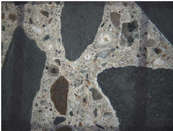
Figure 7.14. A. Highway bridge affected by ASR in Bangor, Maine. Coring sites in the abutment (not exposed (site 1 - B) and the wing wall (exposed (site 3 - C)). D. DRI results for cores obtained from sites 1 to 3; the higher the DRI, the higher the degree of ASR damage in the concrete. E. Polished section from site 1 showing very limited signs of deterioration. F. Polished section from site 3 showing extensive cracking filled with alkali-silica gel in aggregate particles and the cement paste.
