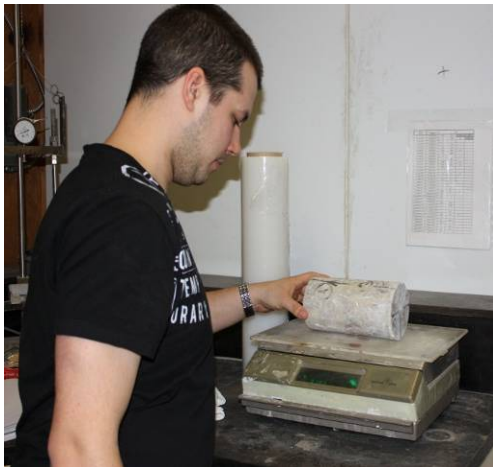
Figure 7.19. Residual expansion testing carried out on core samples (38°C, R.H. > 95%). A. Expansion measurement of the core. B. Mass measurements are also carried out in parallel to the expansion measurements to determine the moisture uptake capacity of the core. C. Example of comparative mass and residual expansion measurements for cores. This allows differentiating the hydric reequilibration of the concrete at the beginning of the test (due to moisture uptake only) and the residual expansion potential due to ASR.
