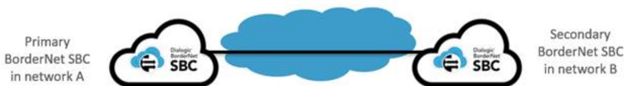
Figure 1: BorderNet in Geo-Redundancy Mode
