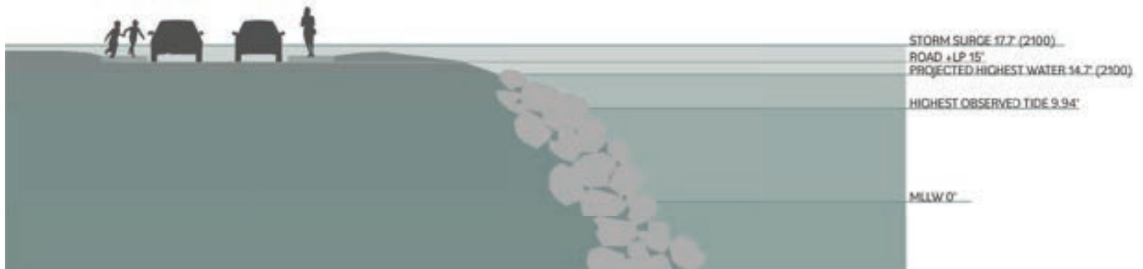
SECTION OF PROJECTED SEA LEVEL RISE IMPACTS ON THE WATERFRONT DISTRICT, INFORMED BY THE BELLINGHAM WATERFRONT DISTRICT SUB-AREA PLAN 2019.
