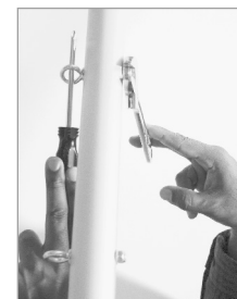
Figure 9: Use two fingers to tighten bolts
