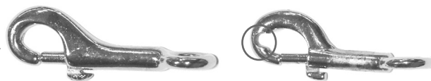
Figure 2: Good snap: no wear on hook. Bad snap: excessive wear on hook.
