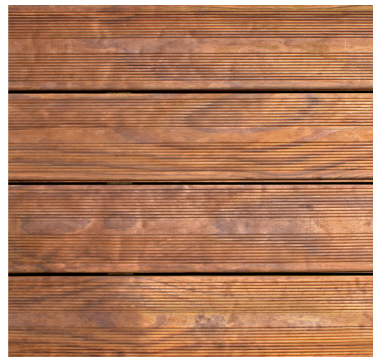
Figure 2: Unfinished Decking material after thermal treatment
