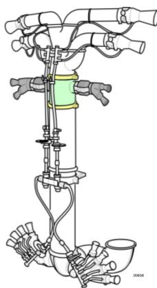
Besides, it is possible to regulate the combined sprayheads' maximum width, by varying the orientation of the "Y" pipe fitting, connecting the main pipe with the diffusers. This solution can result to be especially useful when the rows are particularly narrow.
