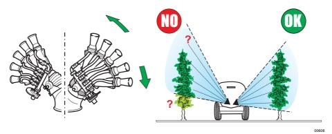
Eventually close the delivery of some diffusers and orient the sprayhead, if the covering angle would result to be too wide.
