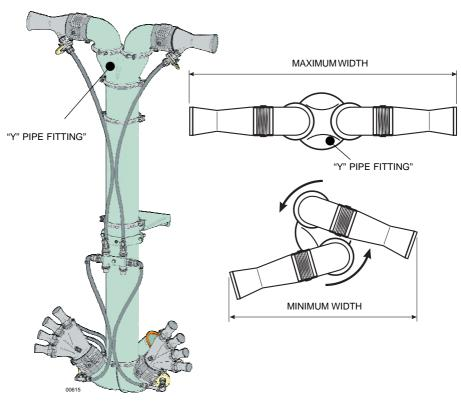
When, on the contrary, it would be necessary to increase the combined sprayheads' upper part width, in order to approach the upper diffusers to the external row, it is possible to use 90° extension elbows longer than the standard ones. The elbows are supplied in a single length version; anyway it is possible to shorten them by following the points foreseen for that operation, in order to reduce them to the wished length.
