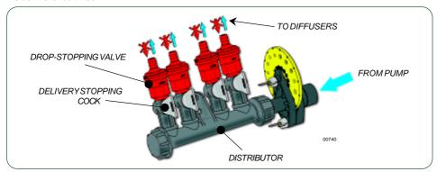
Besides, on the greatest and complex sprayheads, are used valves of different types and materials, they are of the ball-type and of the diaphragm one, used according with the different features of the sprayhead on which they are mounted, and assure the complete absence of losses and droppings, in the full observance of the antipollution rules in force.
