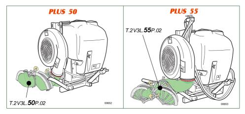
The fixing of the head to the fan outlet mouth (or to the outlet mouth of the fan connecting tunnel, in case of sprayers belonging to the BLITZ series) is realized by means of the fixing collar. In order to better explain how the head fixing is realized, the procedure is illustrated in the following figures; operate in the same way, in order to fix the connecting elbows or the extension tubes.
