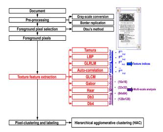
Fig. 1: Pixel-labeling scheme for comparing texture features.
