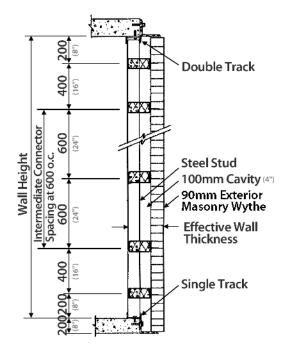
Figure 6 Stud Shear<sup>™</sup> Connector Vertical Spacing
