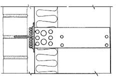
Figure 5 Stud Shear™ Connector Installation
