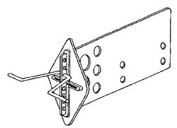
Figure 4 Stud Shear™ Connector (assembled)
