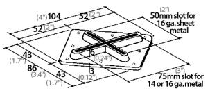
Figure 3 Insulation Support/Retainer
