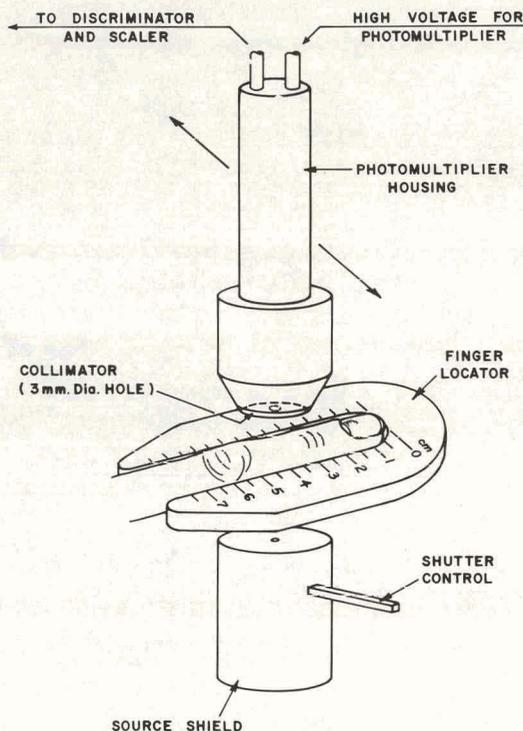
Figure 4. Diagram illustrating the position of finger locator, radiation source, collimator and photomultiplier.
