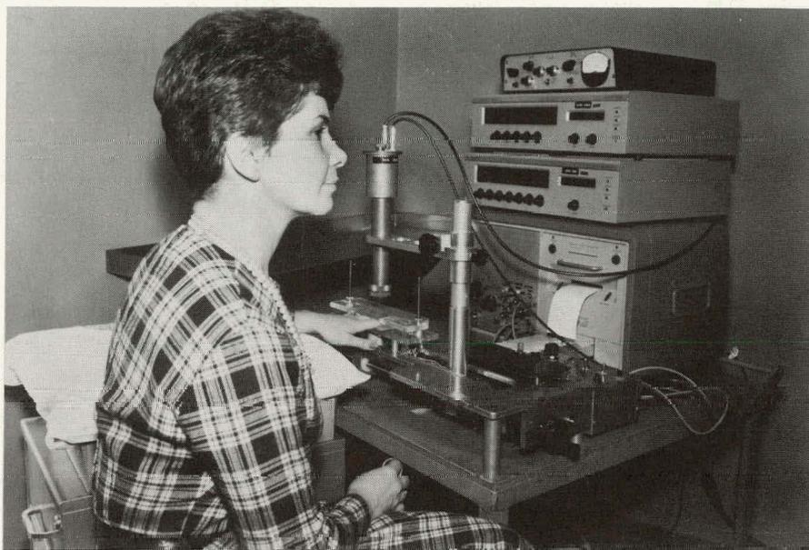
Figure 5. Subject with finger immobilized between plastic plates for counting. Data record appears on paper tape at lower right.
