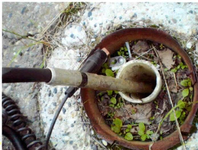
Photo 2. Substance Adhered to Oil/Water Interface Probe
