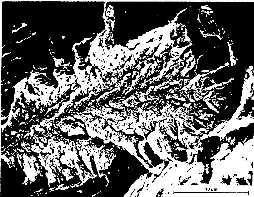
b ROUGH CLEAVAGE FACET WITH MICROERRATED RIDGES
