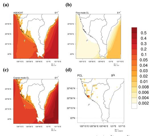
**Figure 2.** CMAQ-calculated (**a**) sea-salt aerosol cation (ASEACAT) emissions (Na<sup>+</sup>, K<sup>+</sup>, Ca<sup>2+</sup>, and Mg<sup>2+</sup>), (**b**) fine-mode chlorine seaspray aerosol (SSA) emissions, (**c**) coarse-mode chlorine SSA emissions, and (**d**) TEDS v10 anthropogenic chlorine (PCL) emissions averaged during the entire simulation period.
