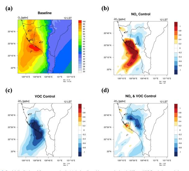
**Figure 6.** Spatial distribution of  $O_3$  concentration in (**a**) the baseline with no perturbations in  $NO_x$  and VOC emissions, and changes in  $O_3$  concentration under the (**b**)  $NO_x$  control scenario, (**c**) VOC control scenario, and (**d**)  $NO_x$  and VOC control scenario at daytime 12:00 LST. All scenarios reduced the targeted emissions by 5 % except for the baseline.
