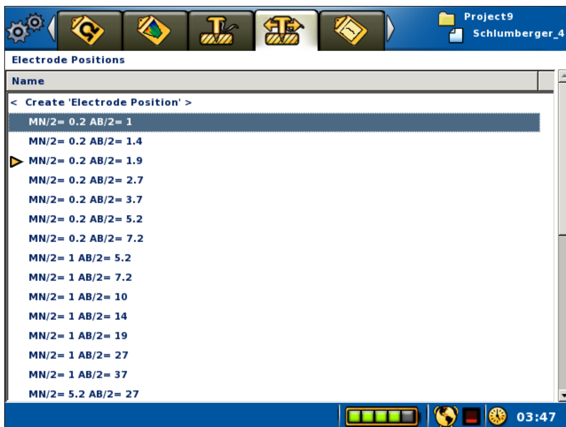
Figure 66 The Electrode Positions view in VES mode. Highlight on the second row and active electrode position marker on the fourth row
