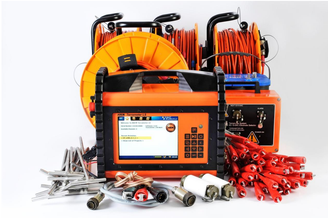
Figure 1 Geoelectrical imaging system with Terrameter LS
