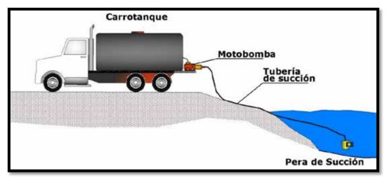
Figure 7.2 Direct uptake system from tank truck Source Gemini Consulting SAS, 2015
