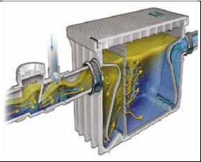
Figure 7.11: Grease trap operation Source Anveplast, 2013
