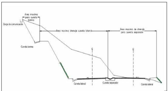
Figure 7.39 Longitudinal drainage elements Source: Consorcio SH
