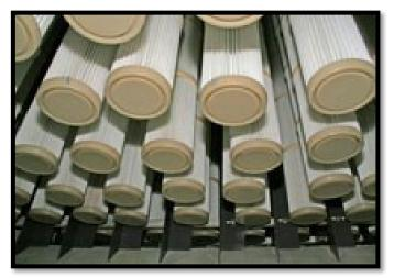
Figure 7.587: Folding sleeves filter Source: (CYBER, sf)
