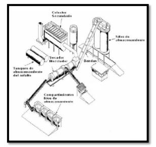
Figure 7.554: Asphalt plant continuous production scheme Source: (States, 2000)
