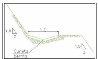
Figure 7.42 Cut berm ditch
