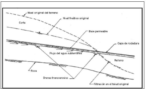
Figure 7.42 Transvers drain on road in cut with perpendicular alignment to existing contour (profile) Source: Consorcio SH
