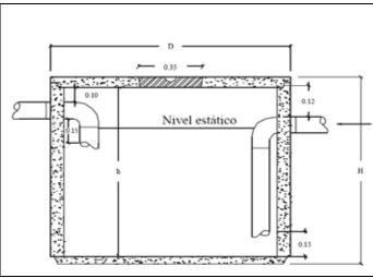
Figure 7.10: Typical grease trap design Source Fatuvisa, 2013
