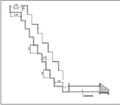
Figure 7.50 Dissipation structure with inlet box culvert Source: Consorcio SH
