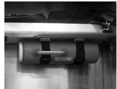
Cylinder straps on a flare container
