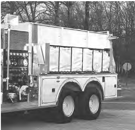
Portable tank in storage position
