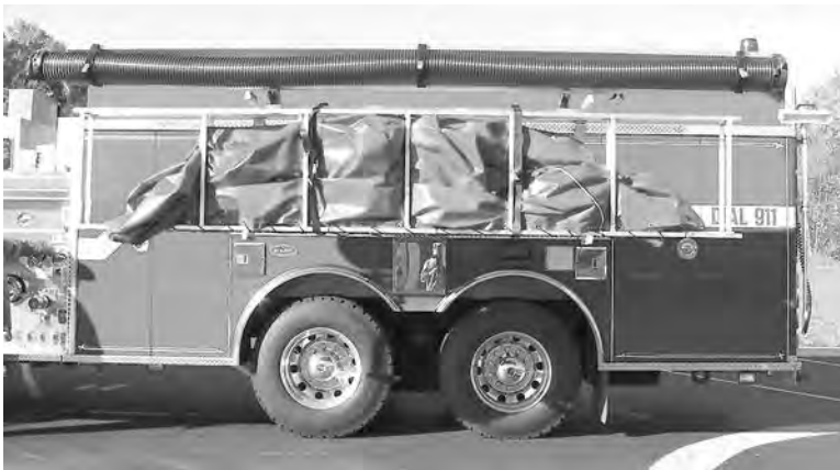
Portable tank lowered for easy removal
