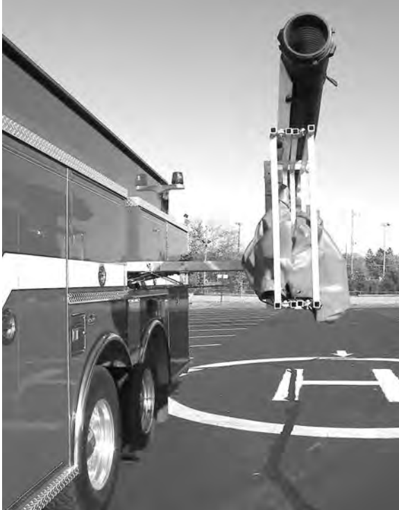
End view of tank and hard sleeve in down position. Compartments remain accessible.
