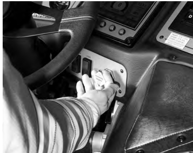
QM-ELB releases upon activation of the parking brake or other 12V switched source.
