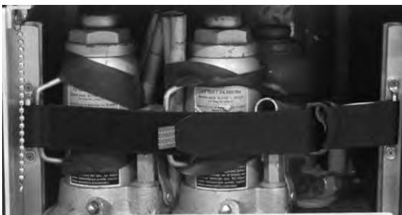
Utility straps securing jacks
