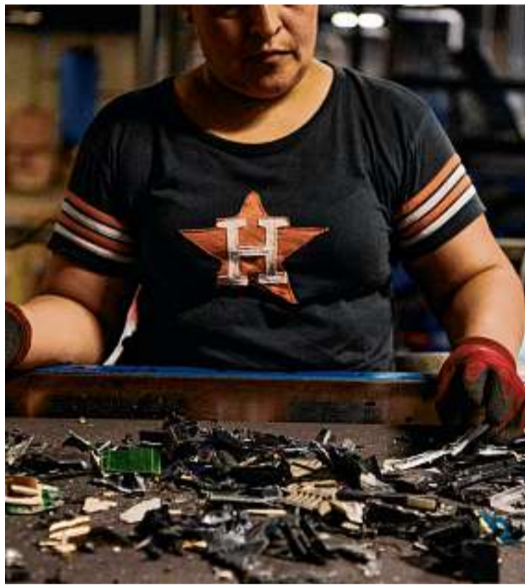
An employee looks for metal pieces among shredded electronics (above). Below, a container of aluminum from shredded devices.
