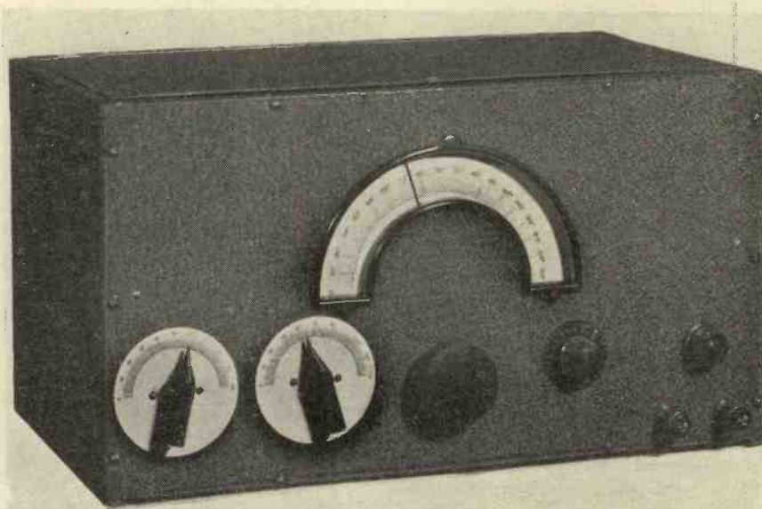
The tuning dial has a travel of 8 in. when used on the 14 mc. band.
