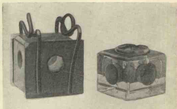
Two more liquid cells made from a glass cube (left) and an inkpot (right)
