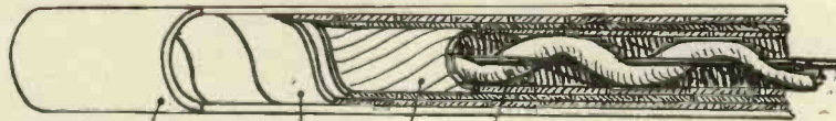
Section of a high-frequency cable; insulation consists of a cotton string wound spirally round the inner conductor.
