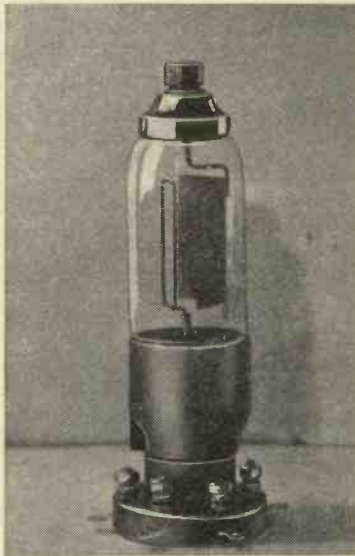
A caesium photo-electric cell of the "plate-cathode" type, suitable for televising films. Commercially produced for talkies.
