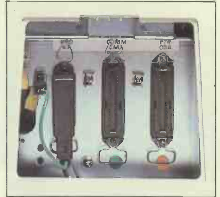
Keyboard connector, comms and centronics printer ports.
