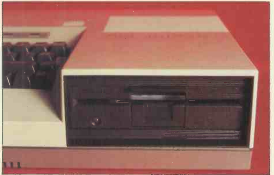
The half-height, 5 1/4 in disk-drive from Mitsubishi is state-of-the-art.
