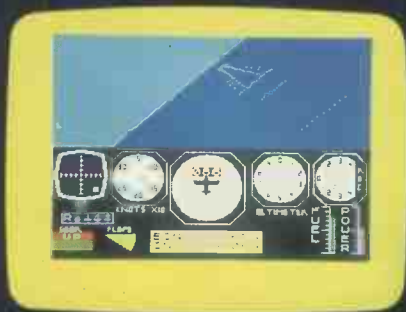
Problem. Simulating an aircraft on a small microcomputer and depicting the 3-D world outside through the eyes of the pilot.
