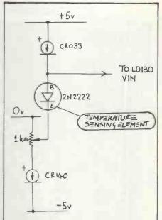
FIG 11. TEMPERATURE TO VOLTAGE CONVERTER.
