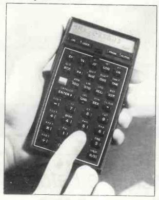
Over 2000 lines of program memory are available or 319 registers. Plug-in modules can be used to extend memory. The HP 41C has a continuous memory and a keyboard which can be customised to users' requirements. Full range of application modules.
