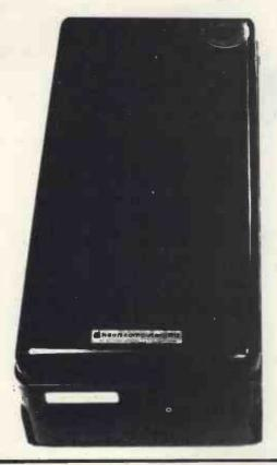
The Corvus 11A hard disk system for the Apple II is made by Corvus Systems Inc. and is imported exclusively by Keen Computers Ltd.
