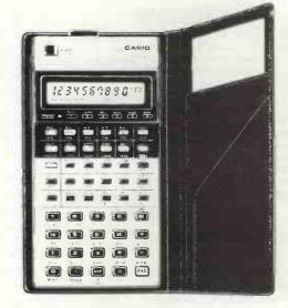
FX-501P. 11 independent memories, 5 level parenthesis, 128 programming steps (non-volatile, 1 step performs a function) FX-502P. 22 independent memories, 10 level parenthesis, 256 programming steps (non-volatile, 1 step performs a function)
