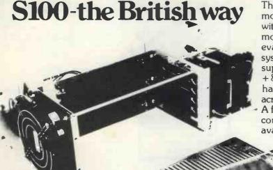
The Vero \$100 Sub Rack is a 19" rack mountable development kit, complete with its own power supply and backplane motherboard, for the construction and evaluation of microprocessor based systems to the \$100 format. The power supply provides three voltage levels -+8V, +18V and -18V. The Sub Rack has its own cooling fan providing airflow across the boards and the power supply. A full range of allied items to enable a complete system to be constructed are available.
