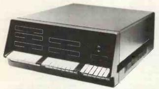
A MINI COMPUTER using MICRO technology at a ridiculous MICRO Price!!! The front panel with a backplane and power supply accepts \$100 bus boards from many manufacturers.
