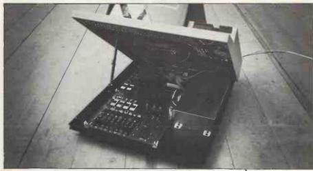
the PET and TRS-80 whereas, if The works...note the sturdy"prop"in comparison, for instance, with that used on the PET.
