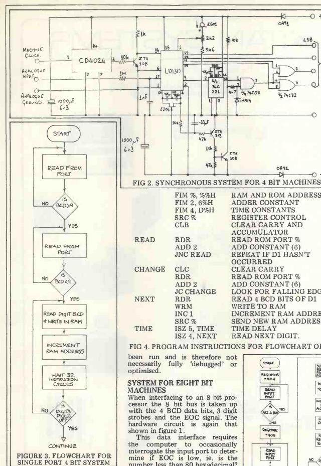
up and stored in memory. D2 and D3 data are picked up 32 and 64 machine cycles later respectively. The flow chart and software for this system are shown in figure 3 and figure 4 respectively.
