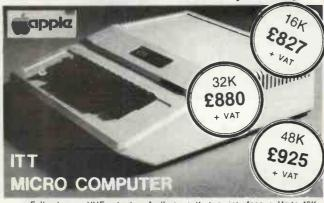
Full colour - UHF output \* Audio cassette tape interface \* Up to 48K RAM on board \* BASIC in ROM (graphics commands include COLOUR = VLIN, HLIN, PLOT and SCRN) \* Built in loudspeaker \* Buckets of software available \* Disk System (110K byte per drive — includes controller) only £425 + VAT EX-STOCK
