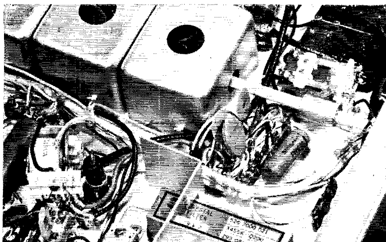
Bottom view of the 75S-3 with relays installed, K_{503} is at the left, mounted on a bracket cemented to the chassis. K_{504} , at upper right, is fastened to the chassis with a machine screw.
