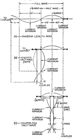
Fig. 1 — Current distribution in three different types of antenna. Note the way the current patterns<sup>a</sup> repeat themselves, but in the opposite polarity, throughout alternate half waves. The dimensions shown are those computed for half-wave antennas operating at 3725 kc., the center of the present Novice assignment in the 3.5-Mc, amateur hand.
