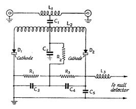
Fig. 5 — Circuit of the phase-angle detector.  $C_1$  — Stray capacitance.
