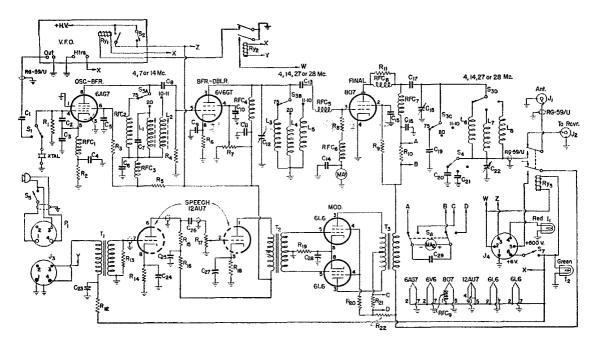
Fig. 1 -- Circuit diagram of the quadriband mobile transmitter.
