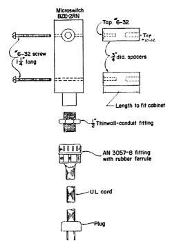
Fig. 1 -Microswitch mounting for service as rackcabinet interlock.
