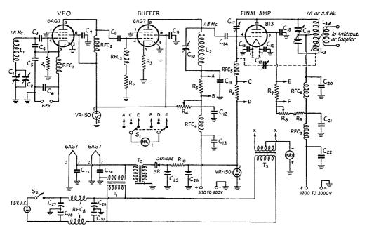
Fig. 1 -- Circuit diagram of the 200-watt 160-meter transmitter.
