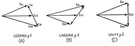
Fig.  $3 \rightarrow$  Relations among secondary voltages in phase-angle detector.
