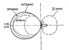
Fig. 2 — Polar diagrams comparing the directive patterns with 135-, 150-, and 180-degree phasing. These figures represent the free-space horizontal-directivity pattern of a horizontal element or array.
