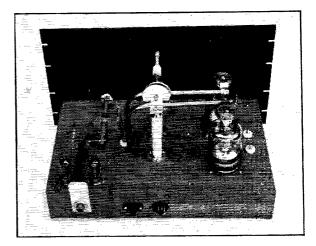
Standard heat-dissipating connectors must be filed down by about one-third of their total diameter, because of the close pin spacing on the 9903. Cardwell butterfly capacitors were selected for  $C_1$  and  $C_2$  because of their provision for ganging. Should these not be available, other types including the Johnson 10LB15 can be substituted by soldering a ganging extension on the rear end of the rotor shaft of  $C_2$ .
