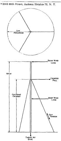
Fig. 1 — Typical mast of the type discussed in the text. For simplicity, it is drawn without the 3- or 4-element beam mounted on the top.
