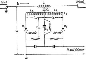
Fig. 1 — Basic circuit of the phase-angle detector.
