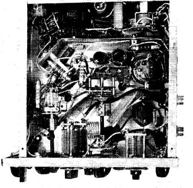
Bottom view of the quadriband mobile rig showing the general arrangement of major components.
