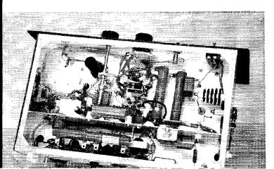
Bottom view of the 160meter transmitter.  $R_4$  is to the left. The inverted 6AG7 oscillator tube is just to the left of the buffer tuning-condenser shaft. In front of the 813 socket are the metershunting resistors and the meter switch.  $R_8$  and  $R_9$  are to the right of the 813 socket. The final plate choke is mounted on the right drop of the chassis. All power wiring is done with shielded wire to suppress v.h.f. harmonics.
