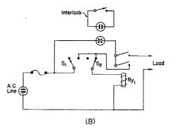
Fig. 2 — A — Simple interlock circuit. The switch is simply plugged in series with the a.c. line. B — Circuit using interlock in conjunction with a locking relay. The switches are push-button type.  $S_1$  (on) is normally open, while  $S_2$  (off) is normally closed.
