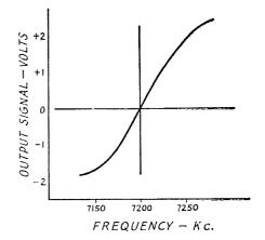
Fig. 4 — Plot of typical output of device of Fig. 5 at a frequency of 7200 kc.
