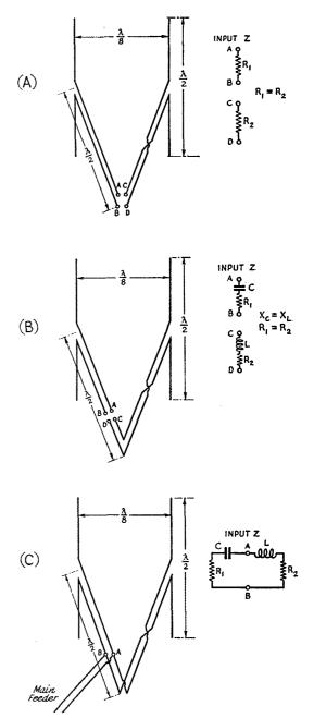
Fig. 3 — Development of the off-center feed method of phasing. The character of the input impedance seen by a transmission line connected to the terminals is shown at the right. As stated in the text, this is based on  $\frac{1}{26}$ -wavelength spacing and exact resonance in each element plus its half-wave feeder.
