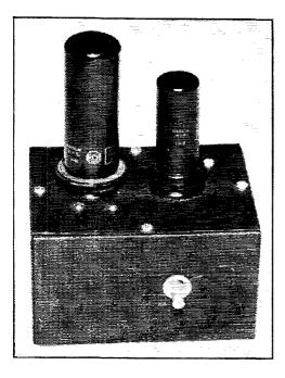
• As W4JJX points out here, a VFO docsn't have to be so elaborate if you are interested in 75-meter operation only. The simple unit described should be entirely adequate for this purpose.
