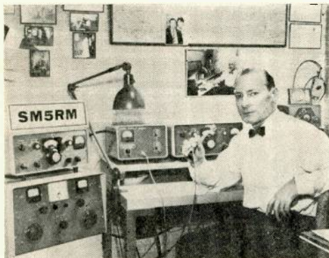
Like many high-power ham operators in North America, Olof Fridman, SM5RM, Stockholm, Sweden uses lots of commercially available gear. The exciter is a Collins Radio 32-S3 which drives a home-constructed linear amplifier. The receiver is also a Collins—a Model 75-S3. Olof is very active on 20, 15 and 10 meters from this fine QTH.
