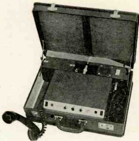
Like CB, portable equipment comes in all sizes and shapes. This "suitcase" transceiver is sold by Aerotron. Battery-operated, it has a 15-watt output.
