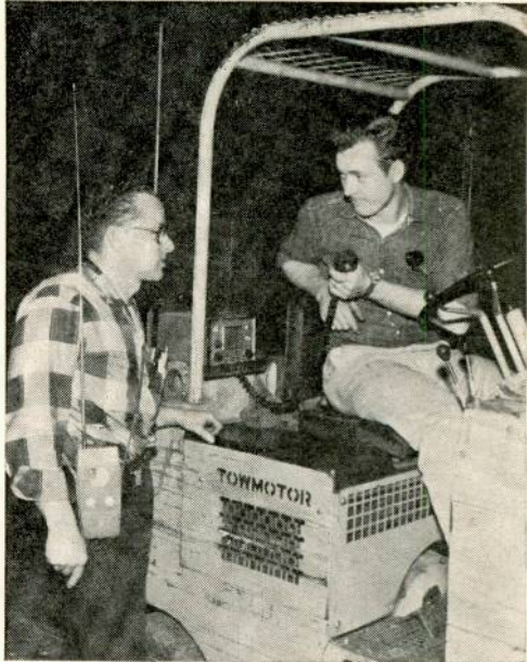
CB has offered the businessman a low-cost method of radio communications. This E. F. Johnson equipment is shown being used at the Charles Machine Works, Perry, Okla. The plant supervisor carries a portable and on the fork lift is a "Messenger I".
