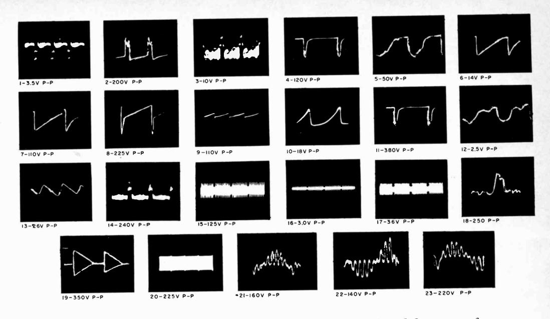
The troubleshooting waveforms shown above have been keyed, by means of numbers, to test points shown circled on schematic. For chroma waveforms, use color-bar generator, wide-band scope with low-capacitance probe.
