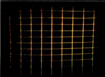
R/G VERTICAL DIFF. AMPLITUDE Converge horizontal red and green lines in the lower portion of the screen.
