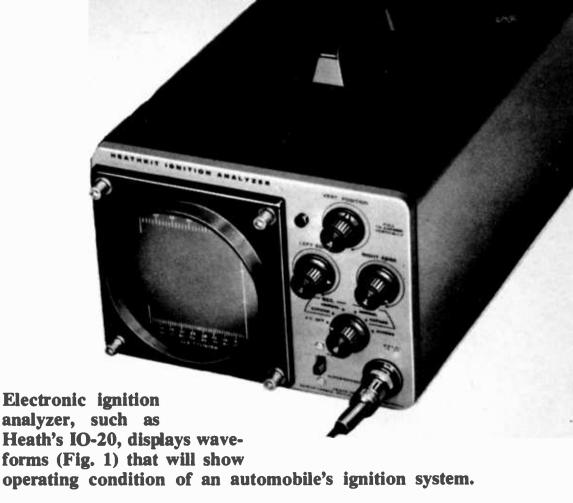
closed-points-and-dwell zone. With the scope graticule calibrated in degrees across the horizontal axis, you can see the dwell angle—in fact, you can adjust the points by the reading.
