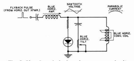
Fig. 8. Blue dynamic horizontal convergence circuit.
