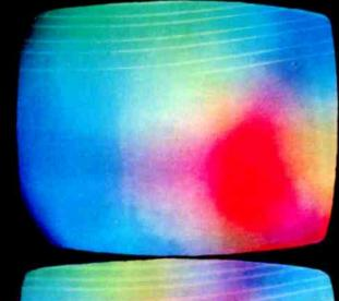
RED FIELD PURITY Set up screen for purity adjustments while operating red gun only with yoke pulled back. Off-centered red spot (top), is centered (above) by adjusting red purity magnet.
