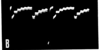
Fig. 6. (A) Stairstep pattern is for checking gray-scale tracking. (B) Waveform shows two "stairs" between each of horizontal pulses.
