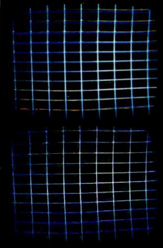
**BLUE VERTICAL AMPLITUDE & TILT** Shift the top and bottom blue horizontal lines up or down to converge with the yellow (red and green) lines to form white lines. Misconvergence is present in both photos. Lower photo shows top lines almost converged.
