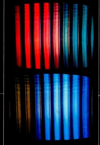
DEMODULATORS INOPERATIVE Defective Z (or B-Y) demodulator shows up mostly as loss of blues (top); predominant loss of reds (above) can be traced to troublesome X (or R-Y) demodulator. Absence of the red or blue colors also causes a loss of the green.
