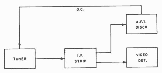
Fig. 4. Closed loop forms automatic fine-tuning system.
