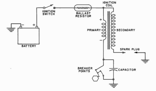
an open circuit between the "+" terminal of the ignition coil and ground. This could be caused by a bad ignition coil, improperly set or dirty points, or an open wiring connection. The source of trouble can usually be isolated by checking continuity with an ohmmeter, or by trial and error substitution of components.
