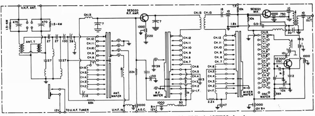
Circuit diagram of the solid-state v.h.f. tuner used in Philco's 19FT20 chassis.
