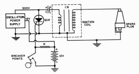
Fig. 7. Simplified schematic of C-D system using SCR.
