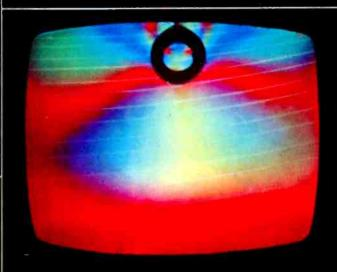
WEIRD COLORS Distortion caused by magnet held close to screen. Use degaussing coil to demagnetize tube and set before adjusting convergence.
