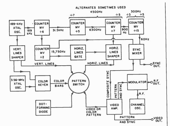
Fig. 1. The basic operating blocks of most color-bar signal generators.
