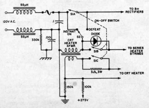
to all tube heaters at all times, even though the set switch is "off," Turning on the switch causes full voltage to be applied to the tubes and also activates the "B+" supply. The entire set comes on almost instantly—within about 8 seconds in the slowest set. Sound is usually a little faster, sometimes preceding the picture by about 5 or 6 seconds.
