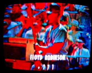
COLOR CONTROL Color intensity should be variable from no color, to washed out color (top, left), to normal (left), to excessive color (above). A little less color is often more pleasing to the viewer than saturated colors.
