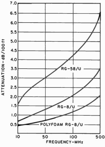
Fig. 3. Attenuation of common coaxial feedline cables.
