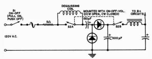
Fig. 6. Manual degaussing system used in a Philco.
