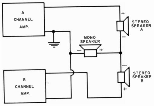
Fig. 3. Novel method of obtaining center mono channel. Special network ahead of amps maintains separation.
