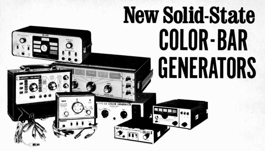
Improved stability, more reliability, longer life, cooler operation, light weight, and portability are the direct result of using transistors and IC's in a new generation of color-bar generators. Here is a complete directory of what's available, along with how the various units operate and compare.
