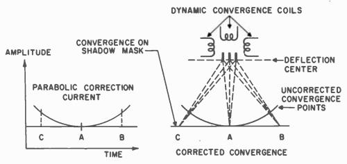
Fig. 5. Parabolic current is needed for convergence.
