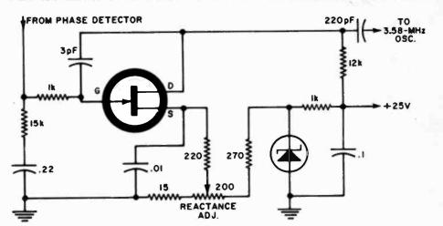
Fig. 2. Junction FET used in Admiral hybrid color-TV set is employed to control 3.58-MHz oscillator.
