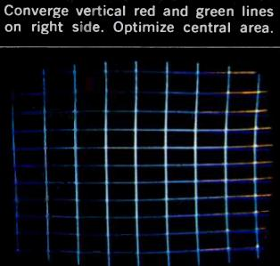
BLUE HORIZONTAL LINES Straighten the blue horizontal center lines to correct droop and misconvergence.
