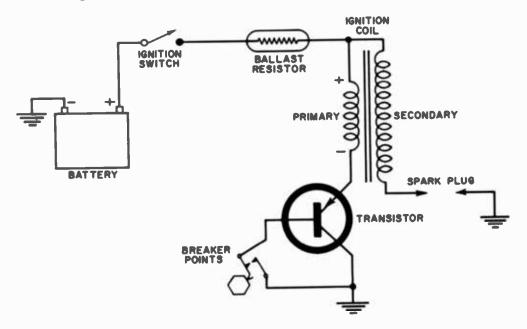
Fig. 3. Simplified schematic of 1-transistor ignition.
