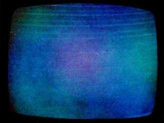
POOR FIELD UNIFORMITY With only the blue gun operating, discolorations due to poor purity adjustments show.
