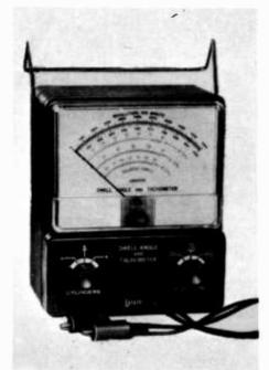
Examples of typical dwell meter (far left) and tachometer (center) are these Delta D-1000 and T-1000. Such units show how long breaker points stay closed, and speed of engine. A combination automotive dwell meter and tachometer (right) is this Lafayette No. 11-0101 unit.
