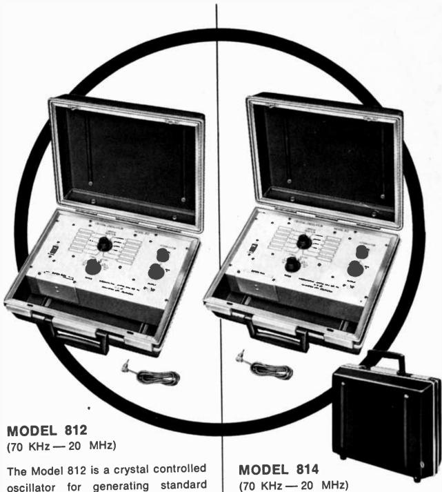
The Model 812 is a crystal controlled oscillator for generating standard signals in the alignment of IF and RF circuits. The portable design is ideal for servicing two-way radios, TV color sets, etc. This model can be zeroed and certified for frequency comparison on special order. Individual trimmers are provided for each crystal. Tolerance .001%. Output attenuators provided. Battery operated. Bench mount available.
