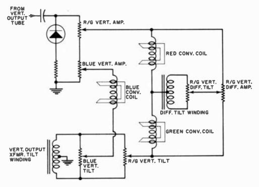
as a start. The blue vertical amplitude is adjusted for convergence with the red/green lines from top to bottom down through the center of the screen. If correction is required at the top because everything from the center down is acceptable, the blue vertical tilt pot may be used to converge blue with red/green lines at top.
