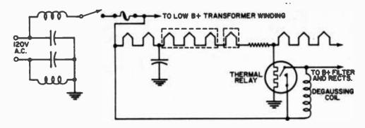
Fig. 5. Some sets use thermal relay to cut off degaussing action before receiver raster comes on. Action of large B + filter capacitor causes current to taper off gradually in degaussing coil before it is shorted.
