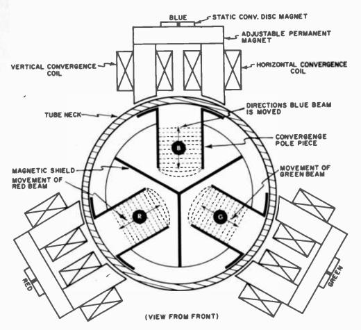
Fig. 2. Assembly for static and dynamic convergence.
