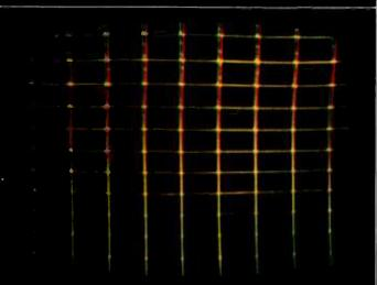
MASTER or R/G VERT. TILT Converge red and green vertical lines at top. Recheck the static convergence.
