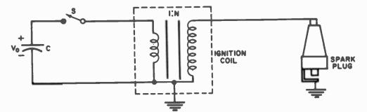
Fig. 6. A simple capacitor discharge circuit and coil.
