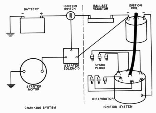
Fig. 2. Arrangement of conventional ignition system.
