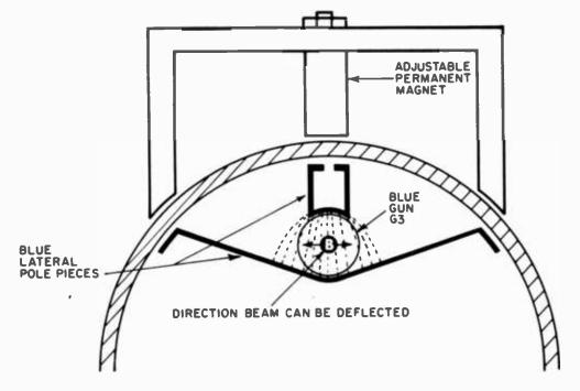
directing the beams to some common point in the center of the screen. Beam-positioning magnets for this purpose are called "static convergence magnets." Older television receivers used d. c. electromagnets; hence, the term "d. c. convergence" may still be used.
