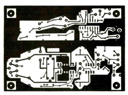
FIG. 3—YOU MUST USE A PC board for the converter. If you don't, the chances are that the circuit will oscillate.
