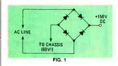
(120 Hz) as it should. You may see one high peak and one low peak, or maybe only one peak at 60 Hz. Here's one example of a problem we ran into. In a fairly old set from General-Electric with separate diodes in the bridge, the sync was affected. That caused some sort of spike voltage that got into the sync circuits and made them false-trigger.
