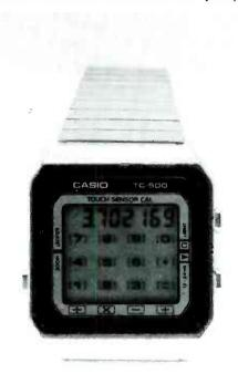
INSTEAD OF KEYS, this calculator/wristwatch from Casio uses a touch sensitive watch face.
