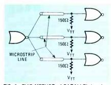
FIG. 8—THIS METHOD of PARALLEL termination uses multiple microstrip lines. The total impedance seen by the gate is 50 ohms.
