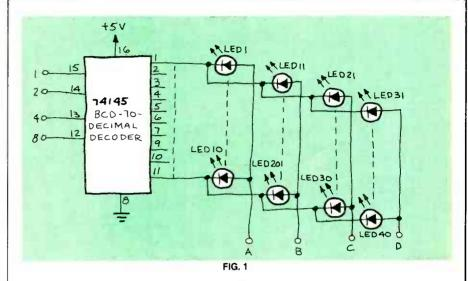
zero to nine. (Only the first and last lines are shown but the other 8 are connected the same way.) Note that each output line is connected to 4 LED's. In addition, one LED in each set is connected to a line (labeled A, B, C, and D).
