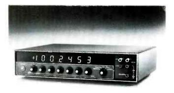
INCREMATIC DC VOLTAGE/CURRENT portable calibration standard allows unlimited use of any one decade with full borrow/carry to and from all more significant digits. This instrument is the model 8200 from Data Precision.
