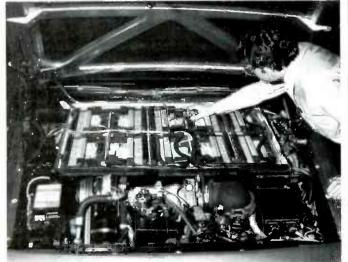
A LOOK UNDER THE HOOD of the experimental "hybrid" electric-gas vehicle developed by General Electric for the Department of Energy shows its stack of lead-acid batteries. Running on electricity for in-town driving, and on gas for the road, it combines the economy and anti-pollution advantages of electric vehicles with the long-range driving advantage of the gasoline engine car.
