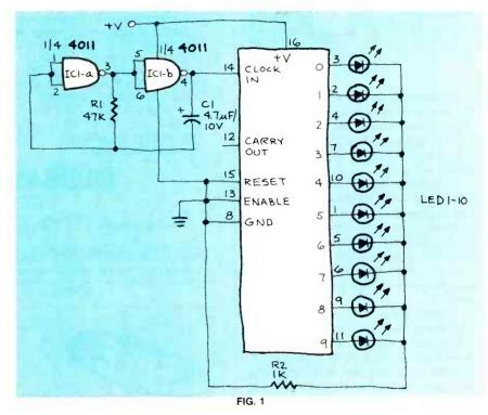
on the RESET pin will make the "0" output go high; it will stay that way until the RESET pin is grounded again. There's also a "carry" output that divides the input clock by ten—it's high for counts zero through four and low for counts five through nine. This IC is really a shift register with a few added bells and whistles. There are, however, some interesting things we can learn from it and some extremely useful things that it can do when we put it to work for us
