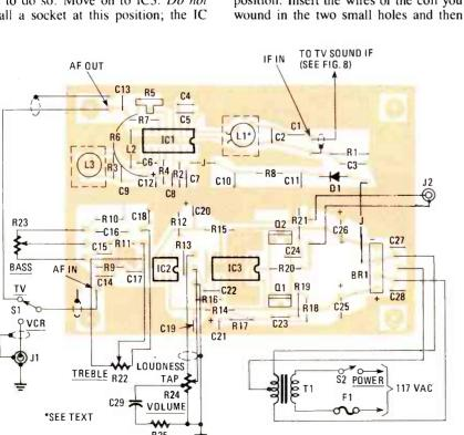
FIG. 4—PARTS-PLACEMENT DIAGRAM. Both on-board and off-board connections are shown.
