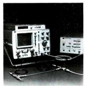
PROPAGATION DELAY CAN BE MEASURED ACCURATELY with the *HP* 1726A time-interval oscilloscope. In this photo a 10-inch length of semirigid coax cable has a delay of -1.43 ns. The minus sign indicates that the channel A signal occurs later than the channel b signal.
