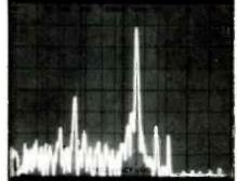
FIG. 9—DISTORTION CHARACTERISTICS for Maxell's metal tape at a 0-VU record level.
