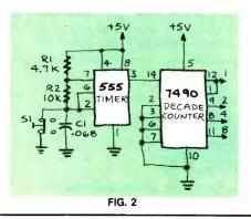
S1. You should not see anything happening; the values of R1, R2, and C1 were chosen to produce fast pulses and the LED's will be flashing so fast you don't see them. As soon as you release the switch, however, the flashing stops and one of the LED's remains on.
