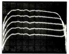
FIG. 3—RESPONSE OF MEMOREX'S TYPE II tape with the recorder set to the T-M BIAS level.
