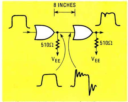
FIG. 1—RINGING IS A MAJOR problem to consider when dealing with ECL-circuit wiring.
