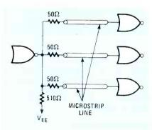
FIG. 10—SERIES TERMINATION using multiple microstrip lines helps to keep power dissipation down.
