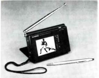
POCKET TELEVISION. This tiny unit from Casio measures 4  $\times$  5  $\times$  1 inches and features a 2¾-inch LCD "screen."
