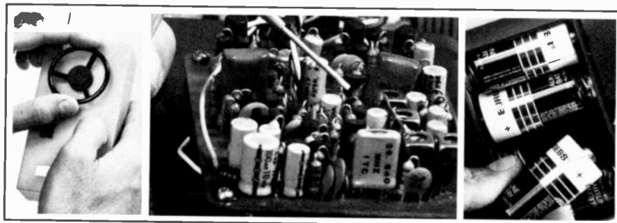
The remote control unit (left) controls the race car's electronics (center). The four "C" cell batteries fit in the underside of the Racer.
