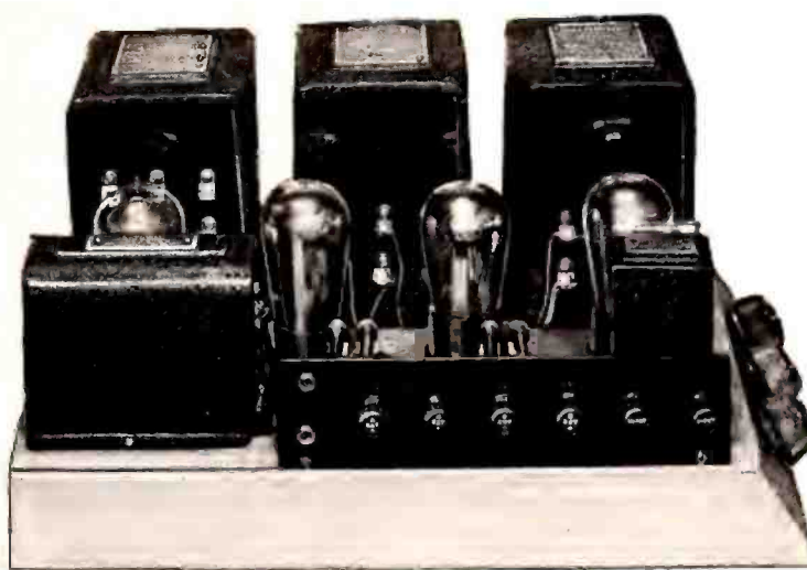
FIG. 3 RADIO BROADCAST Photograph The apparatus is mounted on a substantial cast iron base. The greater part of the wiring is run under this base
