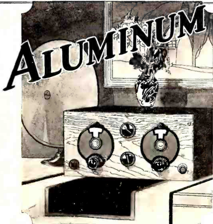
The R. B. Lab. 2-Tube Receiver—is an example of advanced design, with its aluminum cabinet. The aluminum panel combines practical shielding with the beauty of the finest walnut
