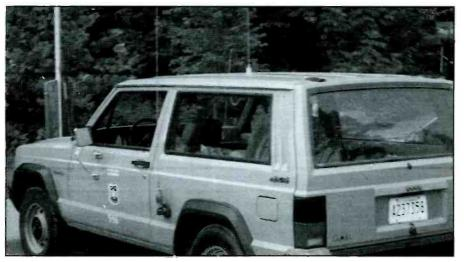
This Dept. of Agriculture vehicle is shown with a VHF high band antenna on the roof. There's also a low band antenna for comms with state and local police.
