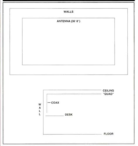
The CB Quad type antenna that you can hang up on your ceiling, after you first construct the thing.
