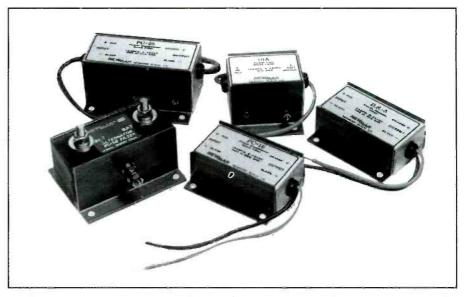
With severe alternator noise, additional filters must be used on the radio siren/PA circuits.
