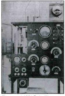
The original 1924 Radio Wien transmitter was a 1.5 kW cabinet job installed in the Ministry of War Building, Vienna.
