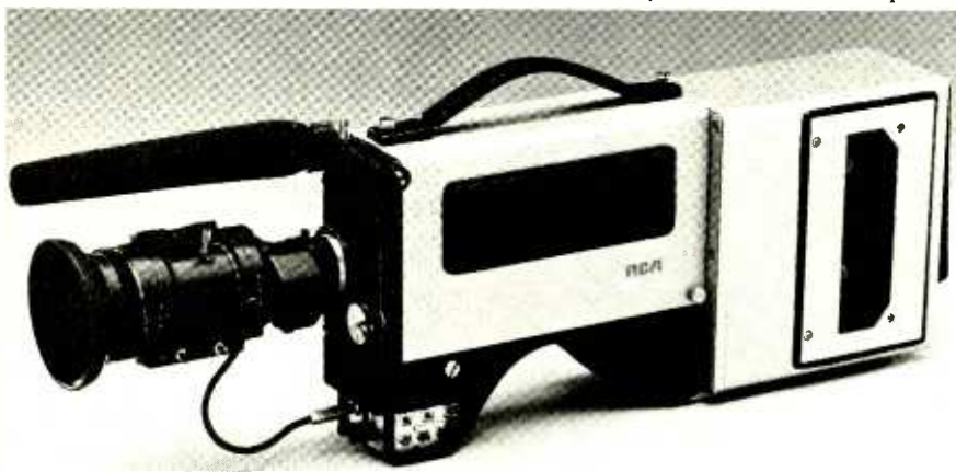
Fig. 1. RCA's Hawkeye Model HCR-1 video camera and tape recorder.
