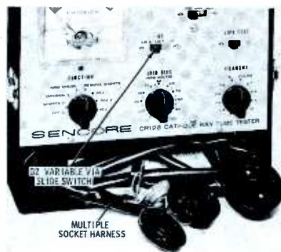
Fig. 1. CRT Tester has provision for three different G2 voltage levels.
