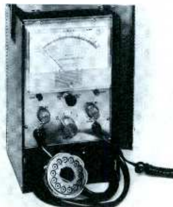
Fig. 4. Color-CRT tester employs two time-based checks for emission quality. ing emission. A pushbutton switch is provided for measuring the quality of the three guns. A red neon indicator lamp shows when power is on, and, as men-
