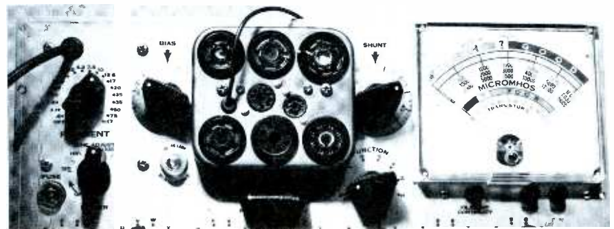
Fig. 4. Separate sockets demount easily by removing two screws.
