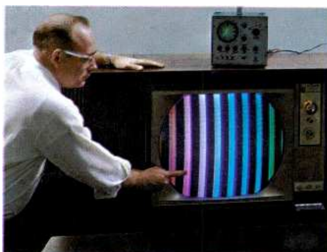
Fig. 2. A 30^\circ phase shift will color third bar magenta.
