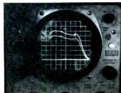
Fig. 13 Video-bandpass response mark is at 8 cm. lower trace 1 db dn.
