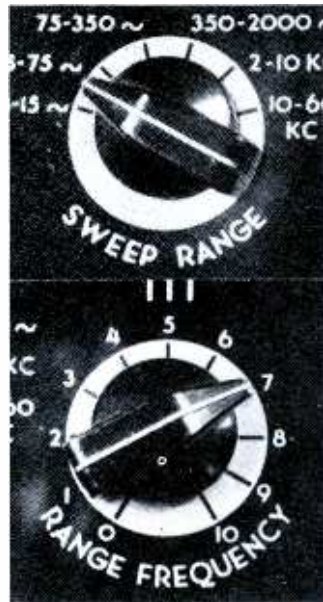
Fig. 6. Sweep-frequency controls for the ordinary service-type oscilloscope.
