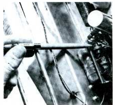
Fig. 9. Peaking coil was mouse food.
