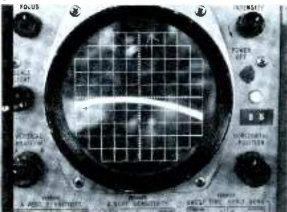
Fig. 5. Scope (calibrated to 1°/cm) shows the differential phase of 1.5°.
