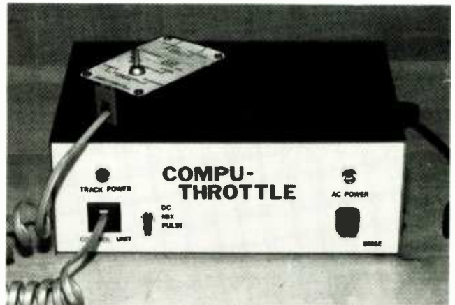
The compu throttle's control cord plugs into the front of the unit using a normal modular telephone cord.
