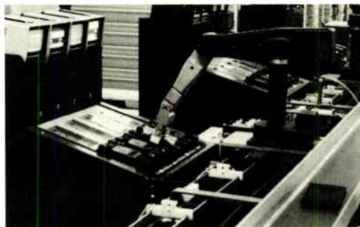
Making money. TI-designed robot places calculators on automatic tester. TI has reduced calculator production costs with this and other automated systems.
