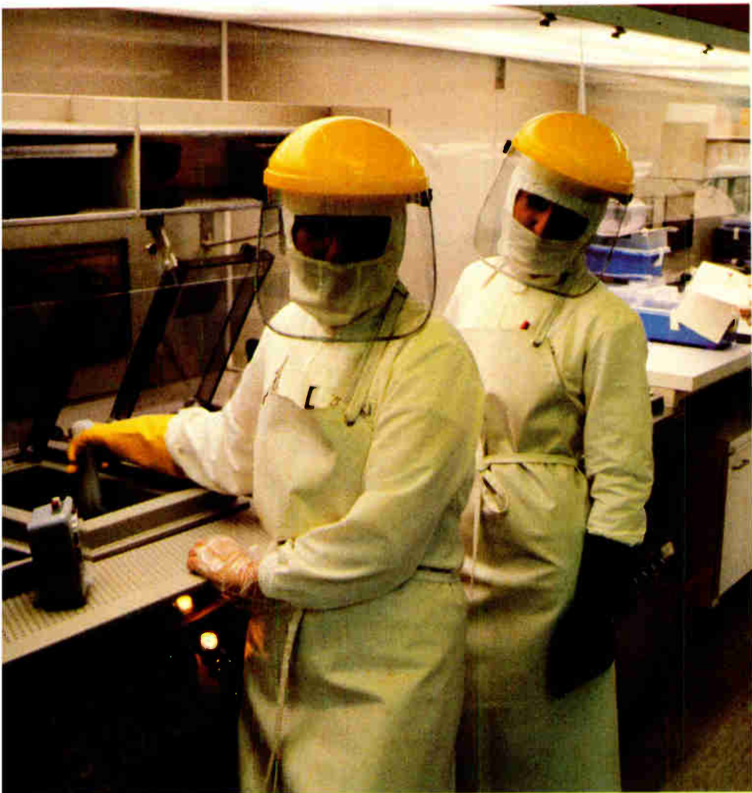
Wet etching of exposed silicon wafers in an ultra - clean atmosphere at Siemens semiconductor plant.
