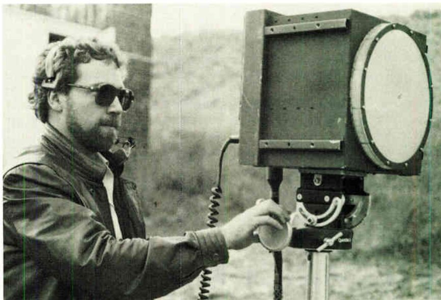
On the air. A member of the Army's millimeter-wave and superhigh-frequency team operates a multichannel command-post radio over a 13-km test link at Fort Monmouth, N. J. The 27-lb advanced development model includes a 10-in. Fresnel lens, as well as GaAs components.
