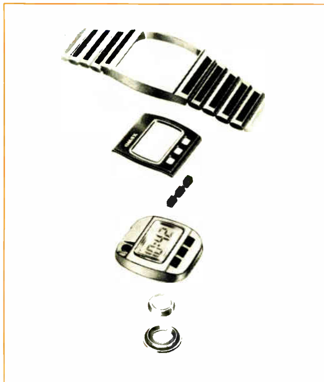
7. Simplicity. This AMI module has command and set buttons on the face and simplified switches to mechanize production, save costs.
