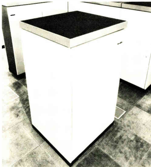
Competitor. This is Intel's in-7168, an add-on for IBM's System/370 model 168. The Intel memory stores 1 to 8 megabytes.
