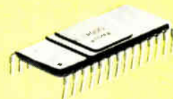
1,021-channel Digital Frequency Synthesizer. 5V supply, 5 MHz input. (HCTR 0320)
