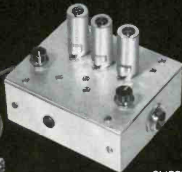
MODEL 100 A TRANSCEIVER WITH NEW DYNAMIC MICROPHONE
