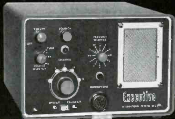
MODEL 100 A TRANSCEIVER WITH NEW DYNAMIC MICROPHONE
