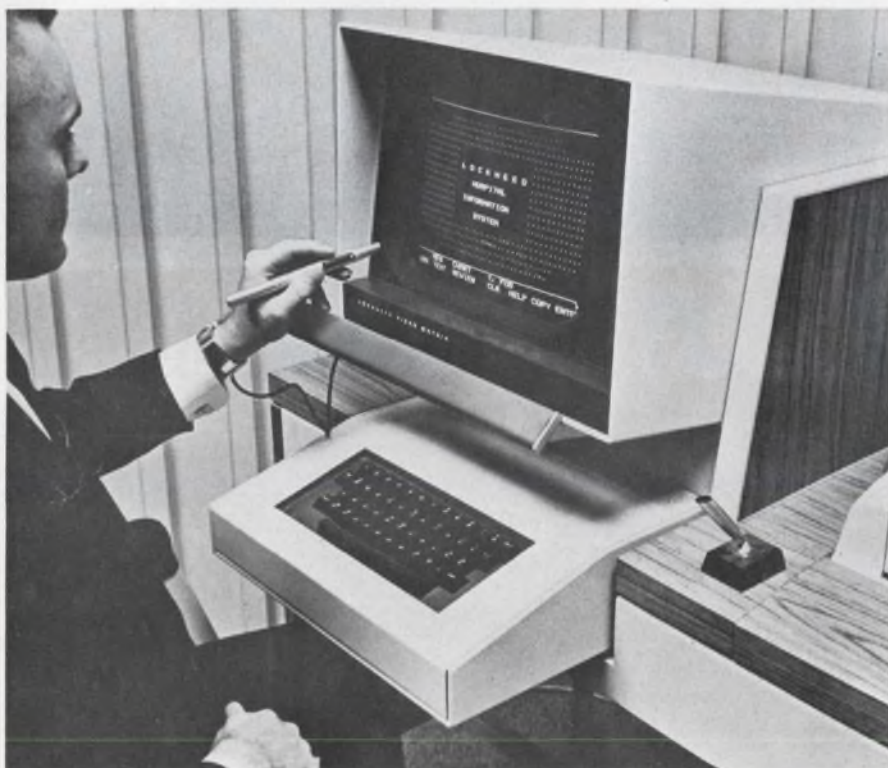
Hospital computer terminal unit is used to issue doctor's orders or check a patient's condition. Light pen summons lists of medical orders to screen. New data are entered on the keyboard, and a printer puts the orders on paper.
