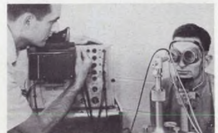
Medical sonar system uses ultrasonic pulses to measure the eye internally.
