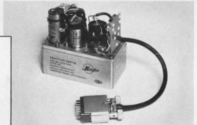
Lead Sight Computer Tracking Servo for helicopter armament system. This servo reflects a special requirement for the command to come from the CT rather than the CX.
