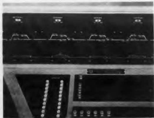
This traffic control center for directing train movements is a good example of the use of backlighting for sophisticated communication with the operator. Here (left) the miniature track diagram contains small backlights that indicate the operational condition of the switches and signals as well as indicator numbers. Backview (right) gives idea of the wiring arrangement used. Union Switch & Signal division of Westinghouse Air Brake was the builder.
