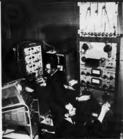
Model I Auditran has tape memory and transistorized light-array output display. Equipment is being used to test envelope detectors and other circuitry and to compile statistical data on performance of the system.
