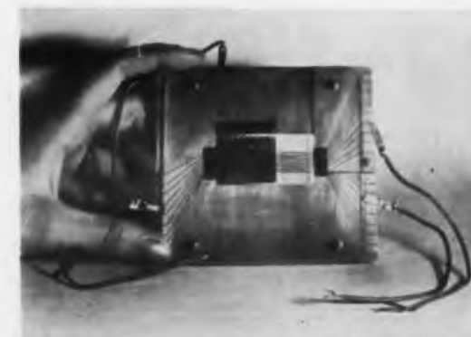
High output voltage of this 64-bit, thin-wall cylinder memory—the Toristor—reduces the complexity of the sense amplifiers, which are similar to those found in conventional, word-organized core memories. CBS Laboratories is working on even simpler circuitry using tunnel diodes as sense amplifiers.
