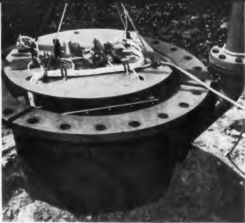
A core of strontium titanate pellets generates heat for thermoelectric conversion to 5 w at 4 v in the unattended weather station. The power charges batteries that drive 250-w transmitters.
