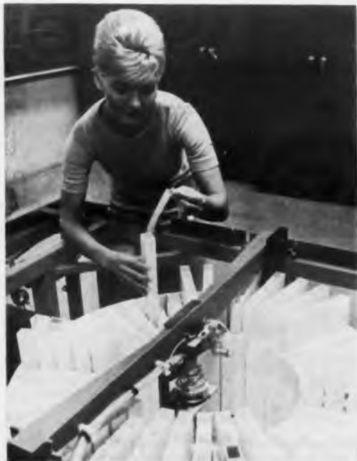
Image file of Walnut Information Directing System, developed for the Central Intelligence Agency by IBM, is made up of 200 plastic cells loaded with film strips. Bin shown contains information equivalent to 3000 books.
