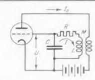
Fig. 66. (a) A tuned-grid oscillator in closed loop form.
