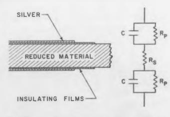
**Fig. 1.** (Above) Physical and electrical models of layerized high-dielectric-constant capacitors.
