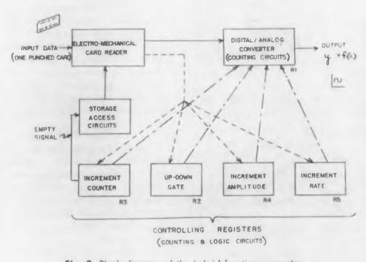
Fig. 3. Block diagram of the hybrid function generator.
