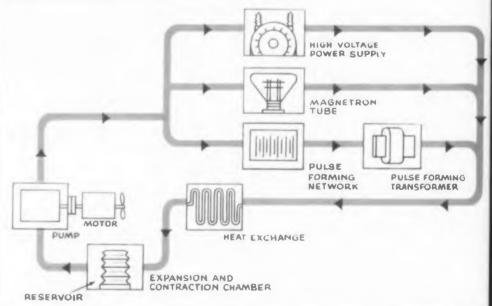
Standardize! Miniaturize! Simplify! Liquid-cooling with Coolanol 45 c help you do all three. The above system design shows one way these thr goals can be achieved when you rely on the fluid properties of Coolanol 4 efficient heat transfer for accurate temperature control...dielectric propert for safe operation...dependable power transmission for the hydraulic tuni circuit. Its complete compatibility with standard materials keeps costs dow
