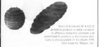
Eccofoam Hi K Flexible Extremely Law Weight Artificial Dielectric Foam Sheet Compressible and flexible. Density about 5 lbs. cu. ft. Temperature range -70 F to = 300 F. For applications which demand low weight, but not structural rigidity. Electromagnetic lenses have been made from this material. It has been used to line the inside surfaces of radomes to adjust electrical wall thickness. It will readily conform to complex contours.
