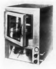
For testing and conditioning transistors, capacitors, and other electronic parts, these vacuum ovens have ambient ranges to 200 and 300 C. Standard units may be equipped with through wall connectors, lead wires, or terminals for the test article, or with doors on both sides of the cabinet for use on production lines. The entire chamber can be seen through the door window.
