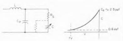
Fig. 3. Parameter values for Hughes diode. Equivalent circuit consists of inductance, stray (parallel) capacitance, series resistance, and voltage variable capacitance. This is a small parallel resistance (dotted lines), but at these frequencies (3000 mc) it is negligible. Curve shows decrease of C with increase of back bias.
