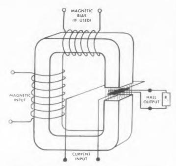
Fig. 5. General electrical and magnetic circuitry.
