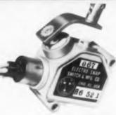
Terminal leads of an Electro-Snap Switch potted in Stycast 2850 GT. The only resin found to completely resist jet aircraft vibration in this landing gear switch application.
