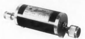
Model – 44 L 1 – 1250-1350 mc 44 S 1 – 2700-3100 mc 44 C 1 – 5200-5900 mc Insertion loss (max) – 0.6 db Isolation (min) – 12 db Power average – 10 w
