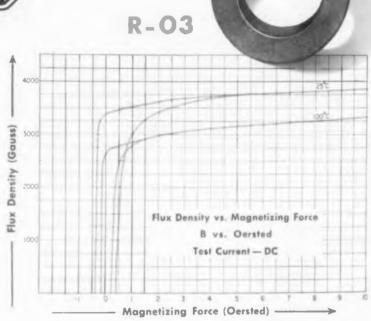
R-03 HYSTERESIS LOOPS show the high flux density provided with low levels of drive. The reduction in area with temperature shows that the loss per cycle is less at higher temperatures. For complete specifications, write for Technical Bulletin 5658.
