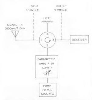
Fig. 1. Typical parametric amplifier. Diode is used as a voltage variable capacitor, inserted in a resonant cavity. Amplified signal is fed to receiver.
