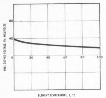
Fig. 9. Hall output voltage vs. element temperature.
