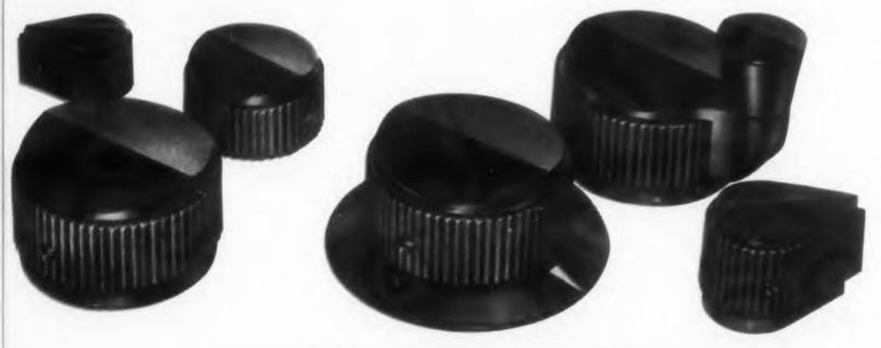
Knobs: Made of plastic, type III, class H2, per Specification L-P-349. Set Screws: Cadmium plated, class 3, type II, per Specification QQ-P-416. Inserts: Brass, composition 4, hard, per Specification QQ-B-613. For price quotations and complete information write:
