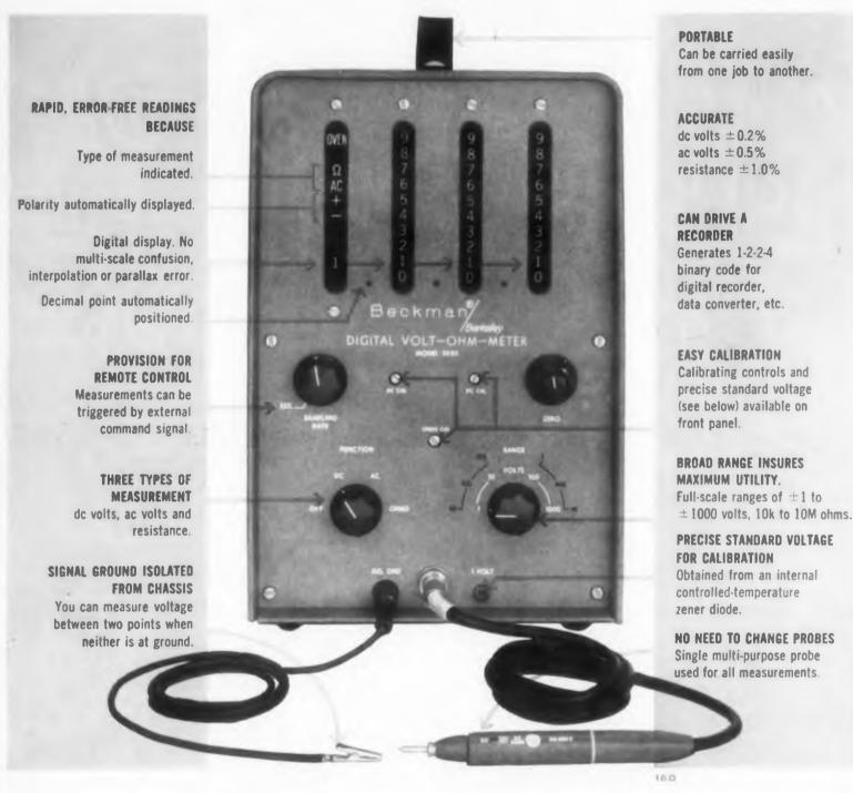
As the picture reveals, BECKMAN/Berkeley's Model 5350 is the most useful, most versatile digital instrument of its kind. It offers operating flexibility and features not found in digital voltmeters costing three times as much. The Model 5350 makes it feasible to replace multipurpose analog equipment with a more accurate, rapid and foolproof means of making the vast majority of everyday voltage and resistance readings.
