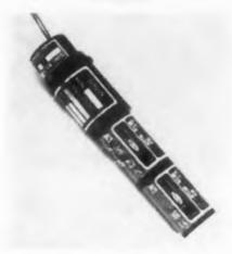
This in-line subsystem consists of a size 10 servo motor, a gear head containing a clutch, and two precision potentiometers. Composed of modular units, the system can be supplied with other motor and gear head sizes. It can also be furnished with any component adaptable to rotary operation, including resolvers, synchros, and tachometer generators.
