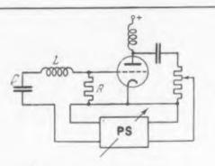
Fig. 59. A typical oscillator with feedback through the tuned grid circuit.
