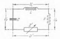
Fig. 61. Equivalent circuit of the resonant circuit of Fig. 59.
