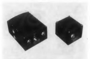
The type 469 high powered C band radar beacon is a pulse type tracking aid for missile applications. The equipment includes a transistorized power supply. It operates over a frequency range of 5400 to 4900 mc and a temperature range of -35 to +70 C.
