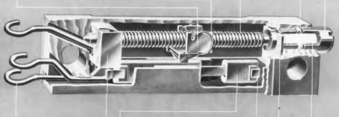
SOLDER TERMINALS — Tinned terminals are compact, yet large enough for easy soldering. Teflon-insulated leads and printed circuit pins are also available.
