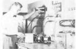
Preliminary testing of foil-wound transformer.
