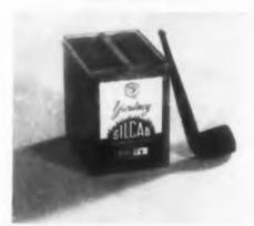
Maintenance free, the Silcad battery is designed to power a completely portable television set. It is also applicable to civilian and military communications systems, to remotely controlled equipment, and to space satellites, where it is recharged by solar cells. A 12 v, 5 amp hr power power package, this silver cadmium battery weighs 3-1/2 lb. It combines the high power output of silver with the long-life of cadmium and can be recycled as many as 200 times.
