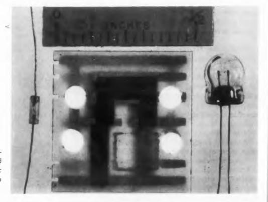
Fig. 1. Two types of miniature indicator lamps compared with 1/2 in. square ceramic wafer (center) containing a printed circuit.
