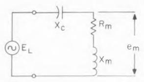
Fig. 2. Fixed phase with a series capacitor to provide 90 deg phase head.
