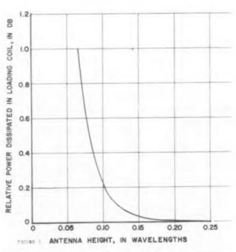
**Fig. 3.** Relative power dissipated in loading coil vs antenna height for a series of inductively-loaded monopoles.
