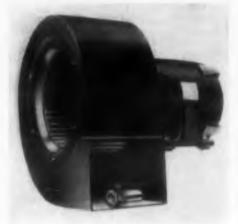
In a wide range of sizes and types, these centrifugal blowers perform a variety of cooling jobs in the electronics and aviation industries. Model FBT 6000B, shown, is a 60 lb unit designed to maintain required ambient temperatures for complex airport ground control equipment. It delivers 2000 cfm at 1 in. static pressure. Miniature model BC 910B, also shown, keeps miniaturized transistor equipment from overheating. This unit weighs 7 oz and delivers 5 cfm at 1 in. static pressure.
