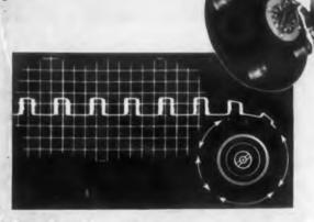
This is one of the many applications for the Stepper Motor — a device for translating electrical pulses into accurate, bi-directional, incremental shaft displacements.
