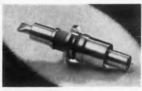
Machlett Laboratories announces the availability of a new ceramic UHF medium-mu triode designed primarily for use in grounded-grid cavity circuits as a plate-pulsed oscillator at frequencies up to approximately 4000 megacycles per second. This new tube also finds application as a radio-frequency power amplifier, continuous wave oscillator or frequency multiplier at frequencies to ap-
