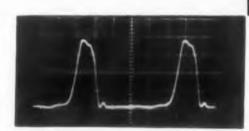
Fig. 4. The pulses, now ready to be delayed, have been amplified by two 6AK5's and two 6888s; voltage is some 75 v, pulse width is 0.53 µsec, rise time 0.12 µsec, fall time 0.14 µsec. Read time from right to left.
