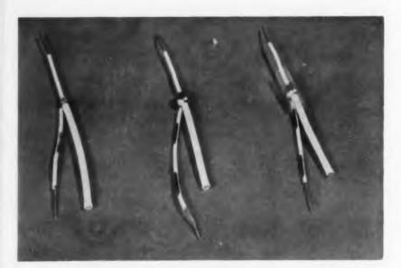
**Fig. 1.** Shielded wire, terminated by casting solder around the connection.
