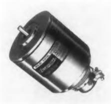
These shaft position encoders are available in true binary, binary coded decimal, and Gray code. They have capacities ranging from 7 to 19 bits binary, and 2000 to 360,000 counts binary coded decimal. Algebraic and transcendental functions are also available. The units have minimum life expectancies of 300,000 to 4 million cycles at speeds to 120 rpm. They have a temperature range of -55 to +85 C and operate under  $\pm 10$  g, 0 to 500 cps vibration.
