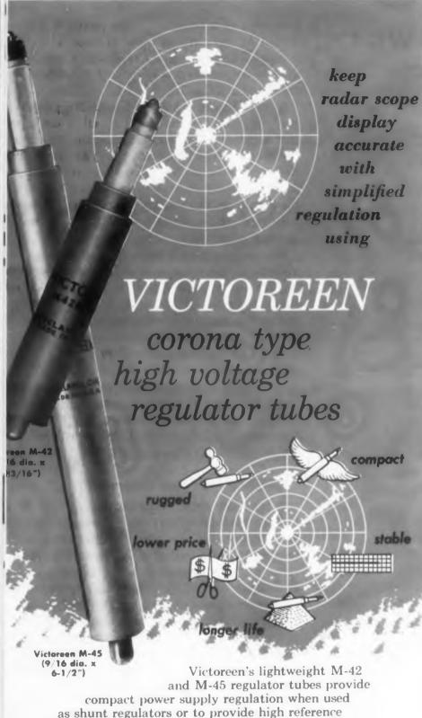
as shunt regulators or to provide high reference voltages for radar scopes and other airborne uses. Currents up to 1mA and nominal voltages from 3kV to 12kV. And, perhaps best of all, experience shows that tube life is considerably longer than that of other forms of high voltage regulation. The complete story on Victoreen M-42 and M-45 Corona Type High Voltage Regulator Tubes is yours for the asking.
