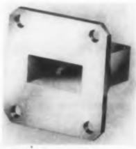
Models 4068-4069 dummy loads and inserts are designed for low power applications. Constructed of vhp material, these terminations are intended to supplant the use of polyiron epoxy resins and other brittle and non-standard terminations. The 4069 series of inserts offers terminations suitably prepared for direct mounting in waveguide. The 4068 series of dummy loads offers the insert already mounted in a short section of waveguide.
