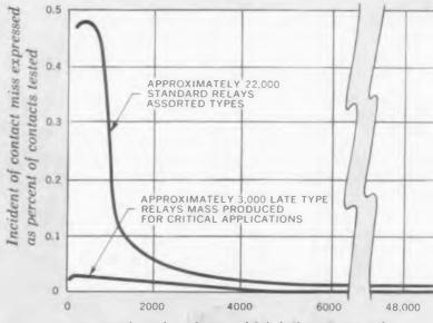
number of cycles at which failure occurred
