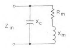
Fig. 1. A servo motor control phase, parallel-tuned for unity power factor.
