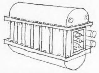
RAYTHEON-DESIGNED, HIGH VOLTAGE DC MAGNETRON POWER SUPPLY
