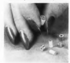
Made of steatite and high alumina, these metallized ceramic diode housings offer good heat dissipation, good thermal and mechanical shock characteristics, and low assembly temperatures. They also eliminate expensive sealing equip-
