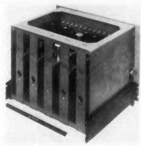
Delay line driver produces pulses delayed some 1.5 usec fifteen times. Pulses remain sharp and square, regardless of condition of input pulses.
