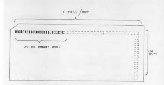
Fig. 1. The basic data card becomes a 78 x 12 storage array.
