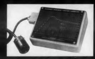
Since different types of pilot balloons have different rates of rise, and wind effects vary with each type of missile, signal inputs to the computer must be easily and quickly adjusted. That's one reason why USASRDL engineers chose two Vernistat Adjustable Function Generators. Only seconds are required to change from one function to another.
