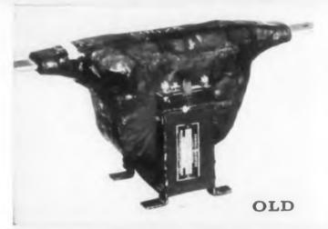
Previous, asphalt-impregnated transformers, made by Canadian General Electric, Limited. Insulation strength was limited.
