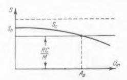
Fig. 70. Average tube transconductance and the feedback function RC/M, both plotted as a function of voltage amplitude for the case where the coefficients  $\alpha_{a}$ and  $\alpha_s$  are negative.
