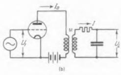
(b) The same oscillator with the feedback loop opened.
