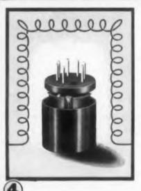
The entire package is then heated; the pellet automatically melts and cures, embedding the component and sealing the cover. In cases where encapsulation is desired without embedment, a self-sealing epoxy cover is available.
