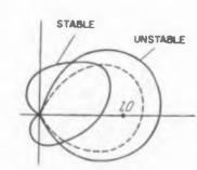
Fig. 65. The amplitude-phase characteristics of stable and unstable systems according to the Nyquist criterion.
