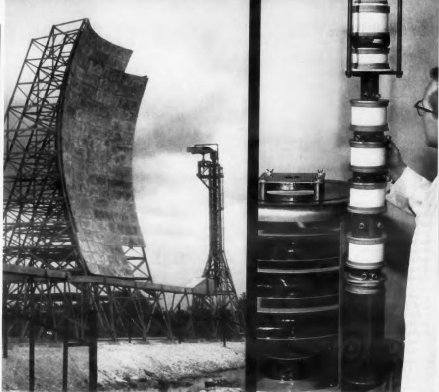
EIMAC Klystrons are used in most trapo-scatter installations
