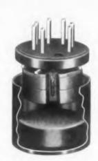
After the component is soldered to the epoxy header, a premetered pellet is dropped into the cured epoxy shell. The cover and component are then inserted into the shell.
