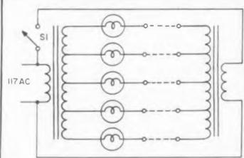
**Fig. 1.** Five wire cable checker. With S1 closed, lamps will light for shorted or interchanged wires.
