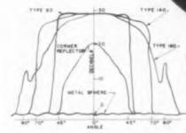
ANGULAR COVERAGE of three types of Ecco Reflectors are compared with a currier reflector and a metal sphere. All are 12" in diameter. Frequency is 9375 mc (3.2 cm). Type 90 Ecco Reflector utilizes... reflective cap which subtends a conical angle of 90. Type 140 subtends 140". Type 180–180. Special caps can be provided for other reflectivity patterns.
