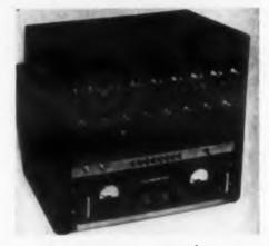
This signal environment simulator generates a realistic high density signal environment in the 200 to 350 mc band, L band, or S band. It simulates eight non-voice radiators, each tunable over a 100 mc range. On all of the eight channels, azimuth bearing of the simulated arriving signal is arbitrary and adjustable. Various antenna patterns may be used on each channel, and each channel has adjustable prf, pulse width, and scan rate. Eight single channel outputs and one mixed output are provided.
