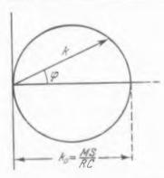
Fig. 67. The amplitude-phase plot of the tuned-grid oscillator of Fig. 66.
