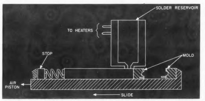
Fig. 2. Casting machine for terminating shielded wire.
