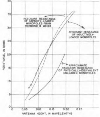
Fig. 2. Resistance at resonance vs antenna height for a series of inductively-loaded monopoles.
