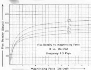
W-07 MAGNETIZATION CURVES show the extremely high flux density available. Also, it reveals that the maximum flux density does not decrease appreciably in increasing temperature. Technical Bulletin 5655 has complete specifications—send for your copy.
