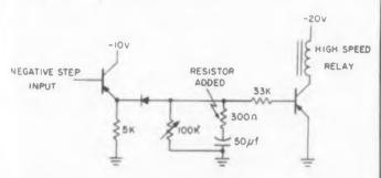
Adding the 300 ohm resistor in series with the iming capacitor allows this long delay circuit to proide very fast attack time.
