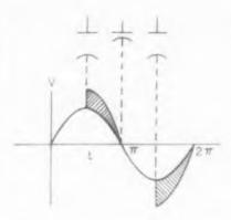
Fig. 2. Principle of parametric amplification. At each maximum of the signal sine wave, capacitance of diode is decreased by applying reverse voltage from klystron. Voltage across diode increases. At  $\pi$  and  $2\pi$  points capacitance increases to nor-
