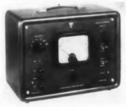
Made by Electronic Instruments, Ltd., of England, the type 33 Vibron electrometer is a vibrating condenser, general purpose de amplifier for measuring small de voltages and currents derived from a high resistance source. Because it neither generates nor absorbs any current from components under test, it can make measurements beyond the capabilities of conventional de
