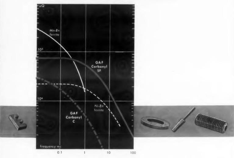
The selection of the proper magnetic core material for the frequency range an inductance coil will be used is of utmost importance.
