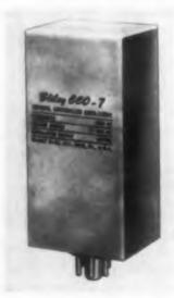
The 1 mc model CCO-7 oscillator provides precise frequency control in a compact transistorized package. Under adverse operating conditions, it has a stability of 4 parts in 10 million. Its features include a glass sealed crystal unit, printed circuitry, and a built-in temperature control. The entire unit is hermetically sealed.
