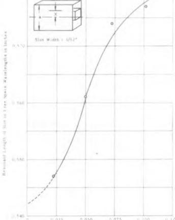
Fig. 14. (right) Longitudinal shunt slots in x-band ridge waveguide. Height = 0.362 in., width  $\pm 0.405$  in.
