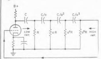
**Fig. 1.** Typical phase shift network in a vacuum tube oscillator has low input impedance, high output impedance.
