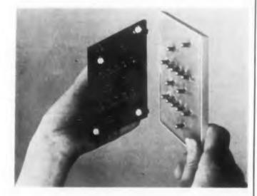
**Fig. 2.** Rear photo of readout lamp showing connector pins and socket. Note shallow depth of combination.
