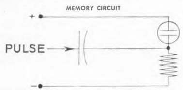
APPLICATIONS—Because of the wide spread between starting and operating voltage, the General Electric NE-96 and NE-97 are well suited for use in switching circuits and counters, where the lamp may function both as the transfer element and an indicator of state or sequence. For full information on G-E Glow Lamps, write for "G-E Glow Lamps As Circuit Control Components". General Electric Co.. Miniature Lamp Dept., Nela Park, Cleveland 12, Ohio.
