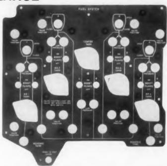
Pilots of Boeing's 707 jet liners rely on new USRengineered fuel system panels for quick, clear, concise information. The ready legibility inherent in the design of these integral edge-lighted panels makes it comparatively simple for the pilot to keep track of fuel load levels in jet flight where fuel management and control are always-critical factors.
