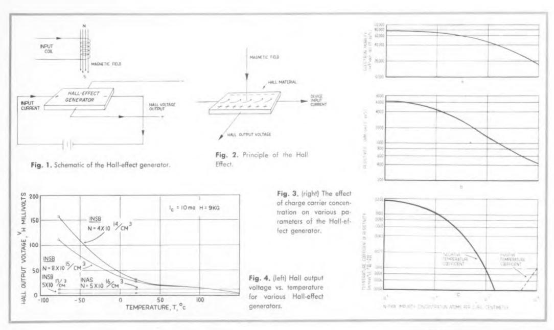
magnetic field to the side of the conducting element. They accumulate there until the force of the electric field created by the accumulating charge balances the force exerted by the magnetic field.
