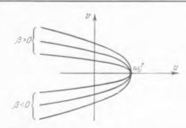
**Fig. 69.** In this hodograph (in rectangular coordinates), when the damping factor  $\beta$  is positive, the system is stable. When  $\beta$  is negative, the system is unstable.
