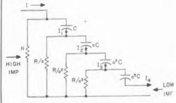
Fig. 2. This phase lead network has a high input impedance.
