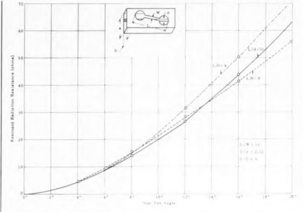
**Fig. 13.** (above) TEM slots in a 70 ohm rectangular coaxial transmission line.
