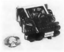
Developed for 400 cps airborne equipment, the model 510-2 transistorized servo amplifier provides an output of 10 w and a voltage gain of 1000. It has an input impedance of 10 K and serves a motor load which requires a 35 to 40 v center-tap supply. The unit employs silicon transistors, measures 2 x 2 x 1 in., and weighs a maximum of 8 oz. It has a temperature range of 55
