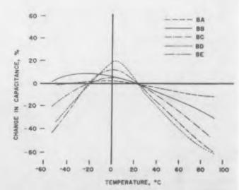
Fig. 4. Per cent change of capacitance of all types vs temperature. Per cent change is calculated from a reference point of 25 C. (Above)
