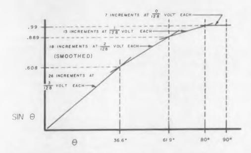
Fig. 2. The first four steps in the linear approximation of a 200 cps sine wave
