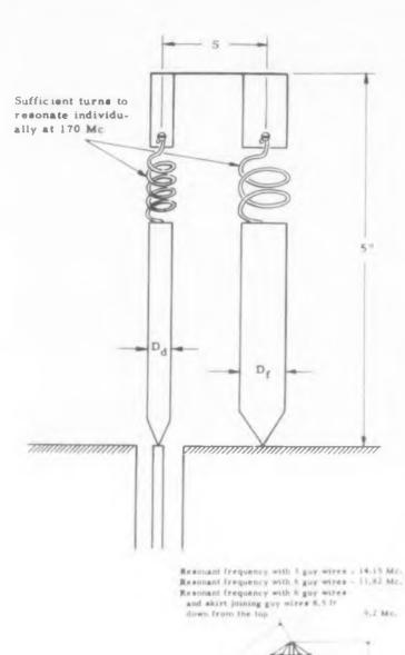
Fig. 5. (above) Capacitively-loaded, folded monopole
