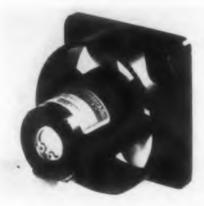
For spot cooling electronic equipment in restricted areas, model S2223-3 tubeaxial fan delivers 40 cfm at 16,500 rpm and 0 in. SP. It has a 1-in. diameter motor and operates from a 200 v, 3 phase, 400 cps source. Built to all MIL-E-5272 specifications, it can withstand ambient temperatures of up to 125 C with a minimum life of 2000 hr. The unit is 2 in. long and has a 2-1/4 in. square mounting flange.
