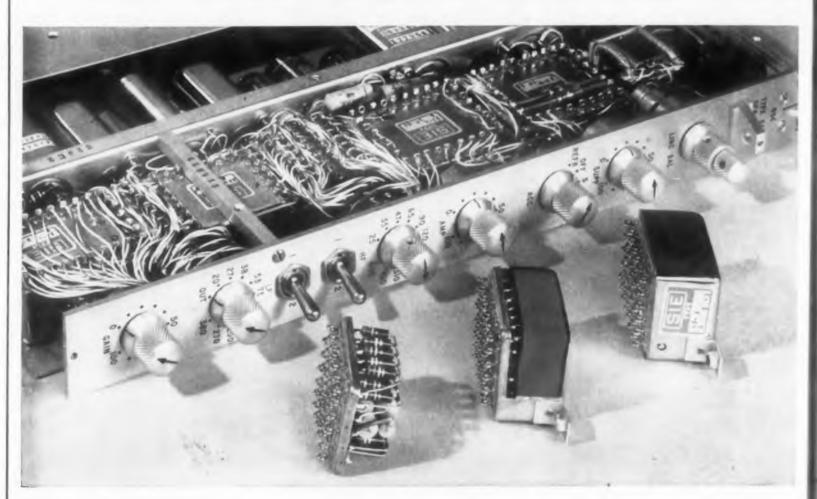
Potted with Silastic RTV, a component can (center) is ready for use in Southwestern Industrial Electronics' geophysical amplifier. Silastic RTV protects and seals circuits against many hazards.
