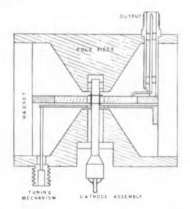
**Fig. 1.** General configuration of a pulsed miniature magnetron.
