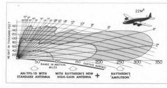
300% increase in coverage and warning time of type AN/TPS-1D radar results when Raytheon's new QK-653 Amplitron and 40-ft. high-gain antenna are added to the system. With other radars of more limited range, improvement factor may be even greater.
