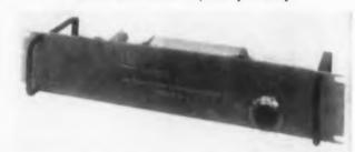
Using a quartz resonator under proportional oven control, the Model RD-146 furnishes a 1 mc output stabilized to better than 1 part in 10<sup>8</sup> per day. The unit has a calibrated trimmer control for making accurate frequency adjustments against crystal aging at various periods without comparison to WWV or other standards. Readability accuracy of the dial is better than 2 parts in 10<sup>9</sup>. Output frequency may be varied and accurately set over 6 cycles.
