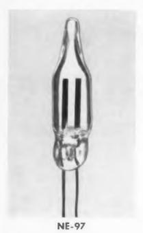
This General Electric NE-97 (and its first cousin, the NE-96) look exactly like the familiar NE-2... but each of these General Electric Glow Lamps has a wider differential between starting and operating voltage. This feature provides a margin of safety against false starting caused by transients in the circuit, since at least a 30-volt pulse is needed to put the lamp in operation.
