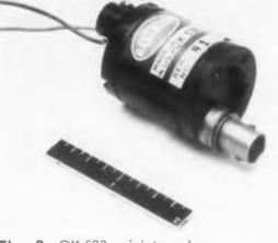
**Fig. 3.** QK-530 miniature beacon magnetron made by Raytheon.
