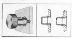
Simplicity of design contributes to clean, distinctive appearance and fast, low-cost installation. Stand-off is slipped into panel hole and secured by flaring. Screw is passed through standoff and made captive by vinyl o-ring.
