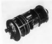
An aircraft panel instrument, this launch range computer solves triangulation problems electromechanically. It is designed to help pilots calculate the distance from aircraft to target and to aid in launching air-to-ground missiles. The unit contains two control transformers, a servo motor, a transistor-magnetic amplifier, a gear train with a slip clutch and pushbutton reset, and an indicator and indicator light. The complete package weighs 44 oz.
