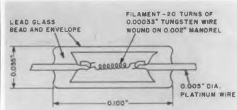
**Fig. 4.** Construction details of early 0.1 in. lamp. Newer lamps are wound with 25 turns of 0.00025 in, diam wire on a 0.001 in, diam mandrel.
