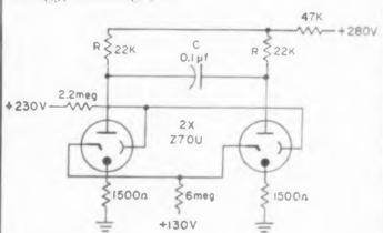
Thyratron oscillator is compact and efficient.
