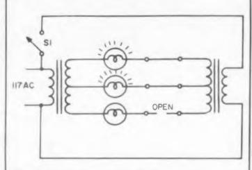
Fig. 2. Continuity check. With S1 open, the lamp in series with an open wire will not light.
