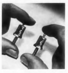
These stable silicon rectifiers are rated at 1500 piv, 300 ma and offer reverse leakages as low as 100 µa at 75 C. Maximum forward voltage drop at 25 C and 150 ma is 4.5 v. Designed primarily for high temperature operation, these units are
