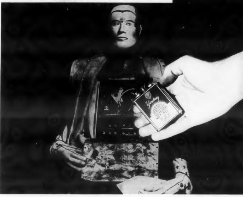
To perfect escape from supersonic aircraft, Coleman Engineering Company, Inc., has created Hurricane Sam, an amazingly real 6-ft., 180-lb. "man". Internally, a YARDNEY SILVERCEL® Battery—a power pack smaller than a human heart—runs strain gauges, accelerometers and a telemetering transmitter, that measure and transmit his almost-human reactions when ejected from a sled traveling at 1,500 m. p. h.
