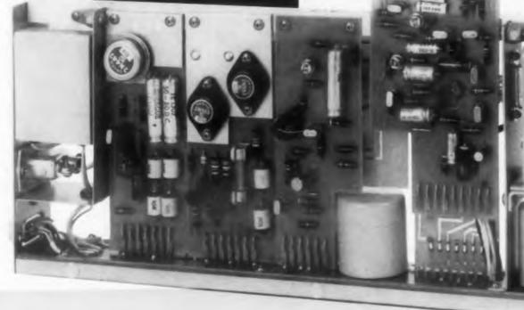
Totally transistorized—dissipates only seven watts.
