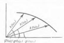
Fig. 64. This amplitude-phase plot shows the locus of the amplitude ratio in the complex plane.
