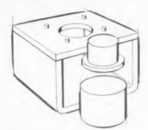
**OLD.** Conventional magnet assembly is larger, heavier, and has a more complex soft steel pole tip.
