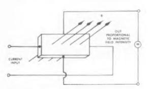
Fig. 12. Magnetic field probe application
