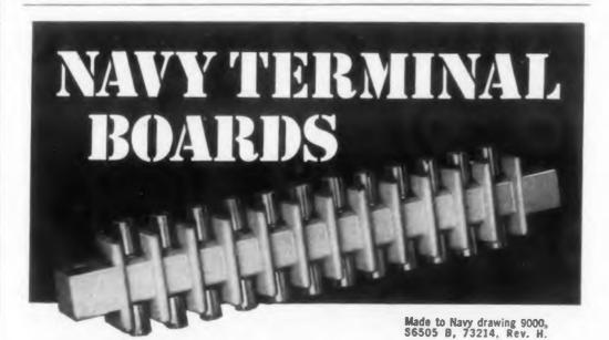
Designed by the Bureau of Ships and covered by applicable MIL specs, these boards or blocks are ideal for other heavy-duty assemblies and services. Available in several different lengths and number of terminals. Supplied in MAI-60 glass-filled Alkyd as per MIL-M-14 with latest revision. Threaded studs of manganese-bronze, molded in plastic. Slotted brass nuts. Other Navy types also available.
