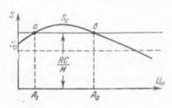
Fig. 71. Average tube transconductance and feedback functions as a function of voltage where the coefficient  $\alpha_3$  is negative and  $\alpha_5$  is negative.
