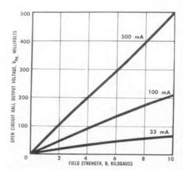
Fig. 8. Hall output voltage vs. Hall output current at various values of magnetic field strength.
