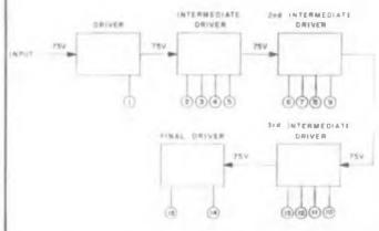
**Fig. 1.** Block diagram of delay line driver. Pulses are amplified and clipped after each 6 μsec. Fifteen output taps through cathode followers provide pulses 1.5 μsec apart.
