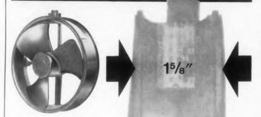
The Saucer Fan represents an entirely new design concept whereby the driving motor is built within the propeller hub limiting its axial length to the minimum measurement required by a highly efficient motor. Ideally suited for tightly packed electronic packages, where space is critical, the Saucer Fan will provide cooling air to the amount of 280 cfm Power requirement is 115 vac. 50-60 cps, 1 Ø.
