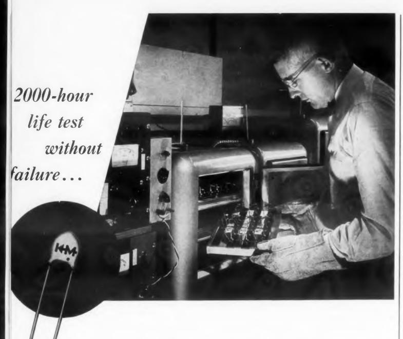
How's this for reliability? After 2000 hours of life test in the ovens shown here—at 85° C ambient, with rated load switched on and off 1.5 million times—new Mallory Type T silicon rectifiers had
