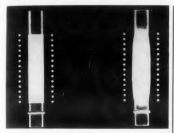
**Fig. 2.** Close dimensional controls are easy with the wrapped cathode (left), very difficult with sprayed cathode.
