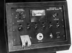
Operates as Go-No-Go Limit Bridge from 100 to 11,111,100 ohms with full scale tolerance selection of 0.01. 0.02, 0.05, 0.1, 0.25, 0.5, 1.0, 5.0, and 10%. Wheatstone Bridge from 1 ohm to 111 megohms. Write for Bulletin P-100.
