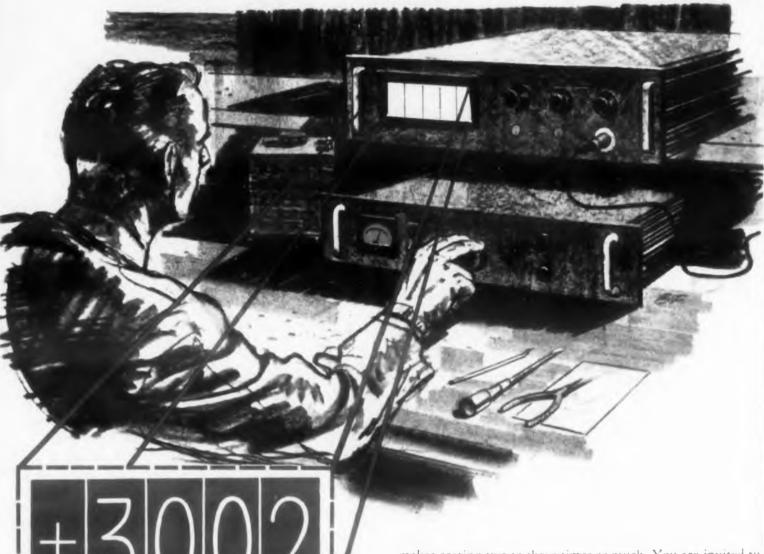
Many manufacturers are finding that power supply testing is greatly accelerated by the NLS 481 Digital Voltmeter. During regulation tests, changes of 0.01% in output voltages are measured and displayed instantly . . . in one-tenth of the time required by manually-operated instruments! As the voltage changes, the 1-inch numerals change on the easy-to-read illuminated readout.
