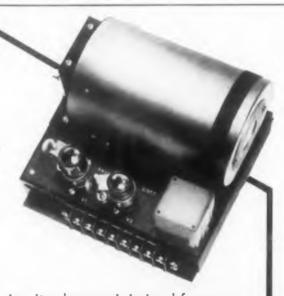
Improvements in the amplifier circuitry have minimized frequency excursions caused by variables such as temperature, plate supply voltage, tube aging, etc.
