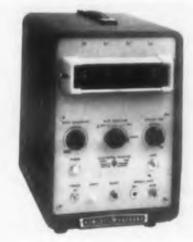
Model 521D industrial electronic counter accurately measures frequency, speed, rpm, and rps, and counts events occurring regularly or at random within a selected period of time. With transducers converting machanical into electrical phenomena, it also measures such quantities as weight, pressure, temperature, and acceleration. The unit features a single line readout and provides a simple conversion to recorder operation.
