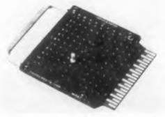
Called the Cross Patch, this printed circuit programming plug-in unit is 4-3/8 x 4-3/4 x 1-1/8 in. It has 11 inputs and 11 outputs which can be interconnected in any combination by inserting banana plugs through the plated-through holes provided. Specifications include operation conditions up to 350 v de at 10 amp with a resistance of 0.01 ohms from input to output. The units can be used at temperatures to 100 C.
