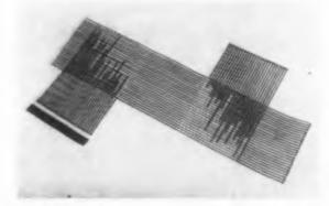
Called Flexprint, this flexible printed wiring can duplicate any wiring cable, harness, or circuit. High density interconnections on the fully insulated flexible matrix are achieved by spot welding of fine etched conductors. These circuits include hookup wire, multiconductor cables with feeder arms, shielded cables, matrix assemblies, and complex, high-component-density circuits. They offer considerable weight, space, and cost savings as well as high circuit reliability.
