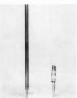
**Fig. 1.** Standard monopole (left) and 0.072 wavelength test monopole.
