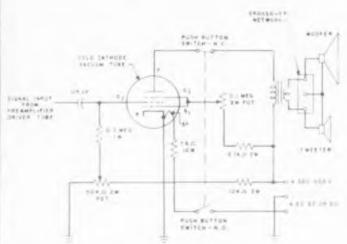
**Audio output** stage using Cold-Cathode Tube, Note high potential on  $G_1$  necessary to sustain emission.
