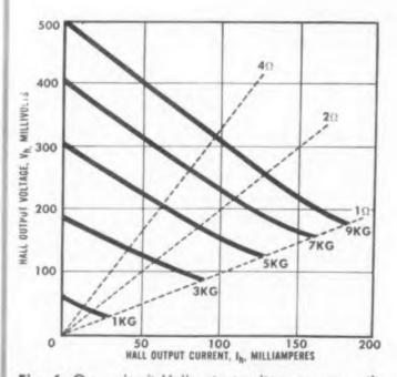
Fig. 6. Open circuit Hall output voltage vs. magnetic field strength for various values of control current.
