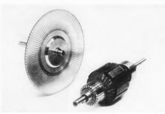
Fig. 1. Because of low mass, the printed circuit armature has a lower moment of inertia than conventional armatures.
