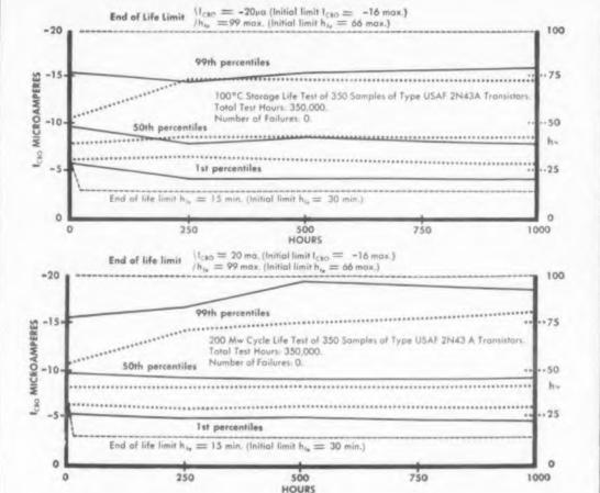
G-E 2N43A LIFE-TEST DATA OBTAINED AT 1000-HOUR POINTS. Upper chart shows results of 100°C storage test (25°C storage test not shown). Lower chart shows results of 200 mw operating test. Broken lines in each chart indicate h<sub>fe</sub>. Solid lines indicate I<sub>cno</sub> in microamperes. After 1000 hours of testing, there were no failures. The 2N43A transistor's high standard of quality is inherent in all G-E germanium PNP audio and switching transistors.
