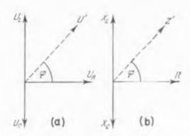
Fig. 60. Voltages and impedances in the resonant circuit of Fig. 59. The phase relationships are shown in (a), while the impedance relationships appear in (b)
