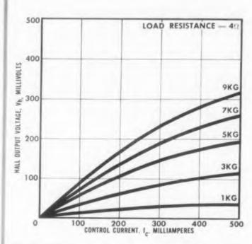
Fig. 7. Hall output voltage into a 4 ohm load, vs. control current for various values of magnetic field strength.
