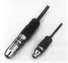
These molded cable assemblies are available in standard 1/4 in. ID sleeve types and in two and three conductor designs. They incorporate types ST-121, ST-125, and ST-131 shielded phone Extension Jax which have OD's of 1/2 and 13/32 in. The units have nickel plated brass housings or sleeves, molded Tenite handles, and paper base phenolic insulation. They are supplied with standard shielded or unshielded cable to desired lengths. Special assemblies are furnished to specifications.
