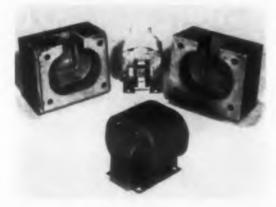
Hysol series 6700 single component epoxy compounds are ready to use without the addition of hardening agents. Stable at room temperature, the compounds meet MIL-T-27B requirements. Filled and unfilled systems are available with several degrees of flexibility and heat resistance to 150 C. The filled compounds are for encapsulation of transformers, toroidal coils, capacitors, and complete circuits. The unfilled are for impregnating transformers and coils.
