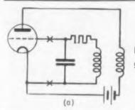
**Fig. 58.** A basic tuned-grid oscillator.
