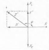
If the absolute value of |R'| is greater than R, the system becomes self-excited. As to X', as can be seen from the diagram, its presence is equivalent to increasing the inductive reactance X<sub>k</sub> (or reducing the capacitive reactance  $X_c$ ).
