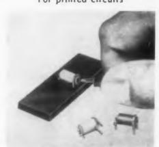
The Press-Fit SKT-103 PC miniature jack mounts flat against a printed wiring board. It has a double-prong steep strap in front, and a connection lug in back which fit in three small holes forming a triangle in a grid coordinate layout. It is dip soldered from the underside of the board for mechanical and electrical requirements. Made with a self-aligning Teflon hole, the unit takes a 0.08 in. probe with no strain on the contacts.
