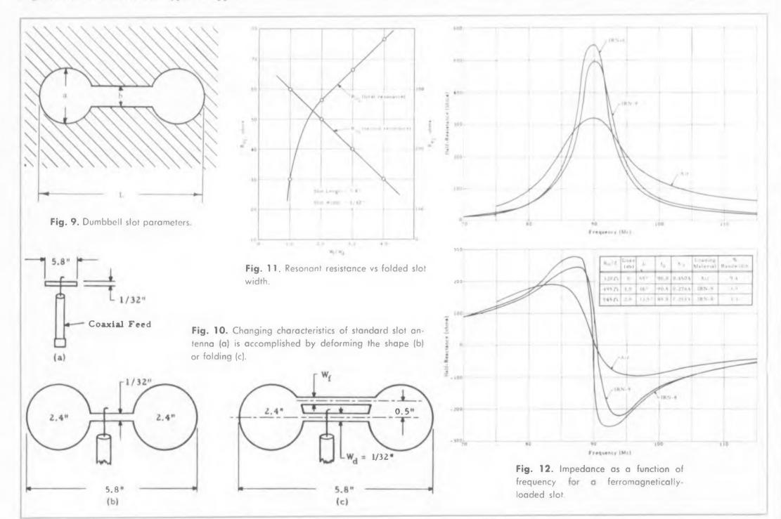
reducing the length of the slot antenna and making compensating changes in the electrical characteristics are suggested by considering methods which have been used with linear antennas.
