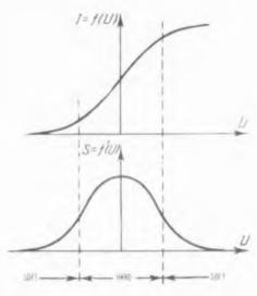
**Fig. 72.** Boundaries between hard and soft modes of oscillations are determined by points of inflection of the characteristic of the transconductance.
