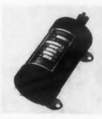
Designed for use with the company's continuous cable aircraft fire detection system, the model 297-115-3 magnetic amplifier control assembly is 1-3/4 in. in diameter and 3-5/32 in. long. It weighs 0.8 lb. Ruggedly constructed, it does not require a shock mounting and can be placed almost anywhere in the aircraft. The unit consumes 1 w for either standby or alarm and will carry a load of 170 ma at 28 v dc. Controls capable of carrying larger loads are also available.
