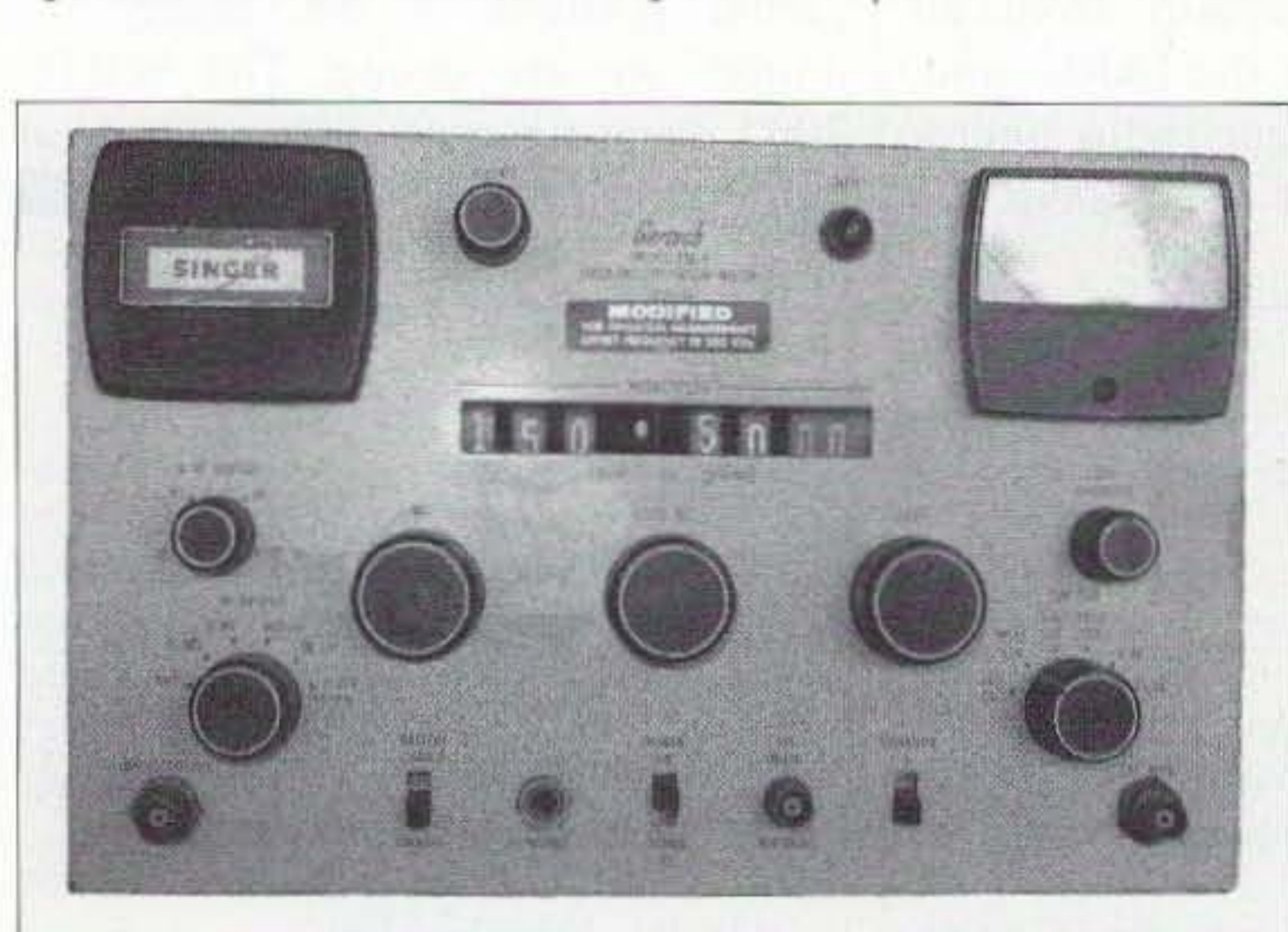
Photo A. A front panel view of the Singer-Gertsch FM-9 frequency/deviation meter.
