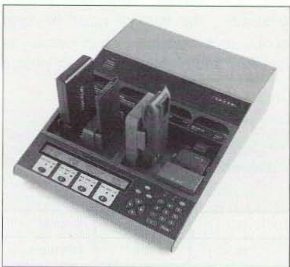
Photo A. The Cadex 7400 programmable four-station battery analyzer has a range of 1.2 V to 16 V and 100 mA to 4 A. Each station operates independently. Custom battery adapters simplify battery interface; universal adapters accommodate less-common batteries. Nickel-based batteries are automatically reconditioned if the capacity falls below the user-defined target capacity.
