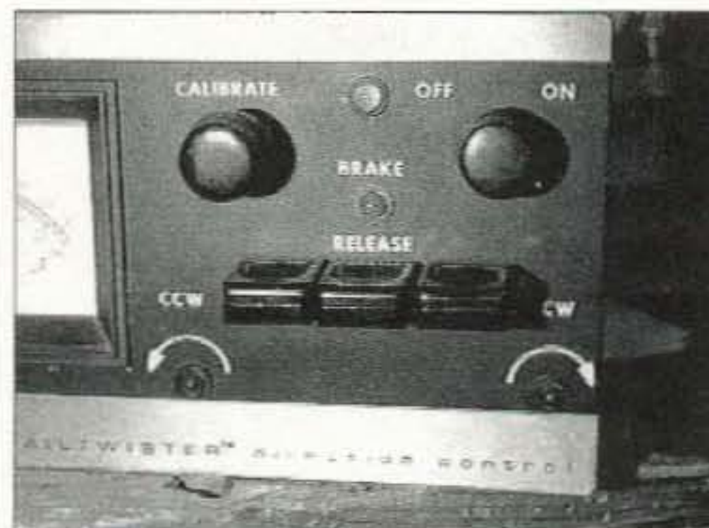
Photo F. The added LED shows between the two knobs and above the original BRAKE RELEASE LED.
