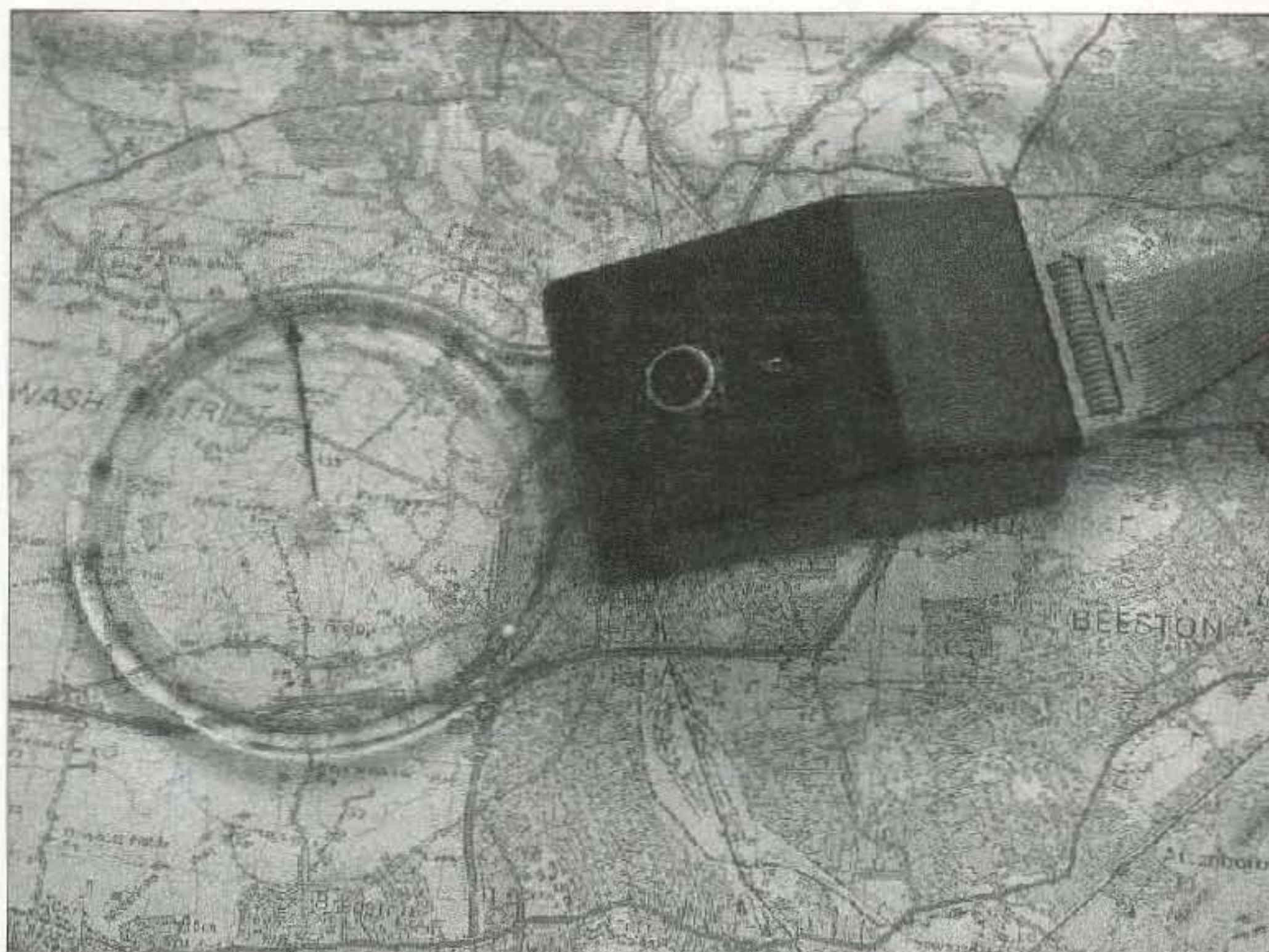
Photo D. Transferring bearings from display to map is easy with this wand of light-emitting diodes. (Photo by Dave Bullock G6UWO)
