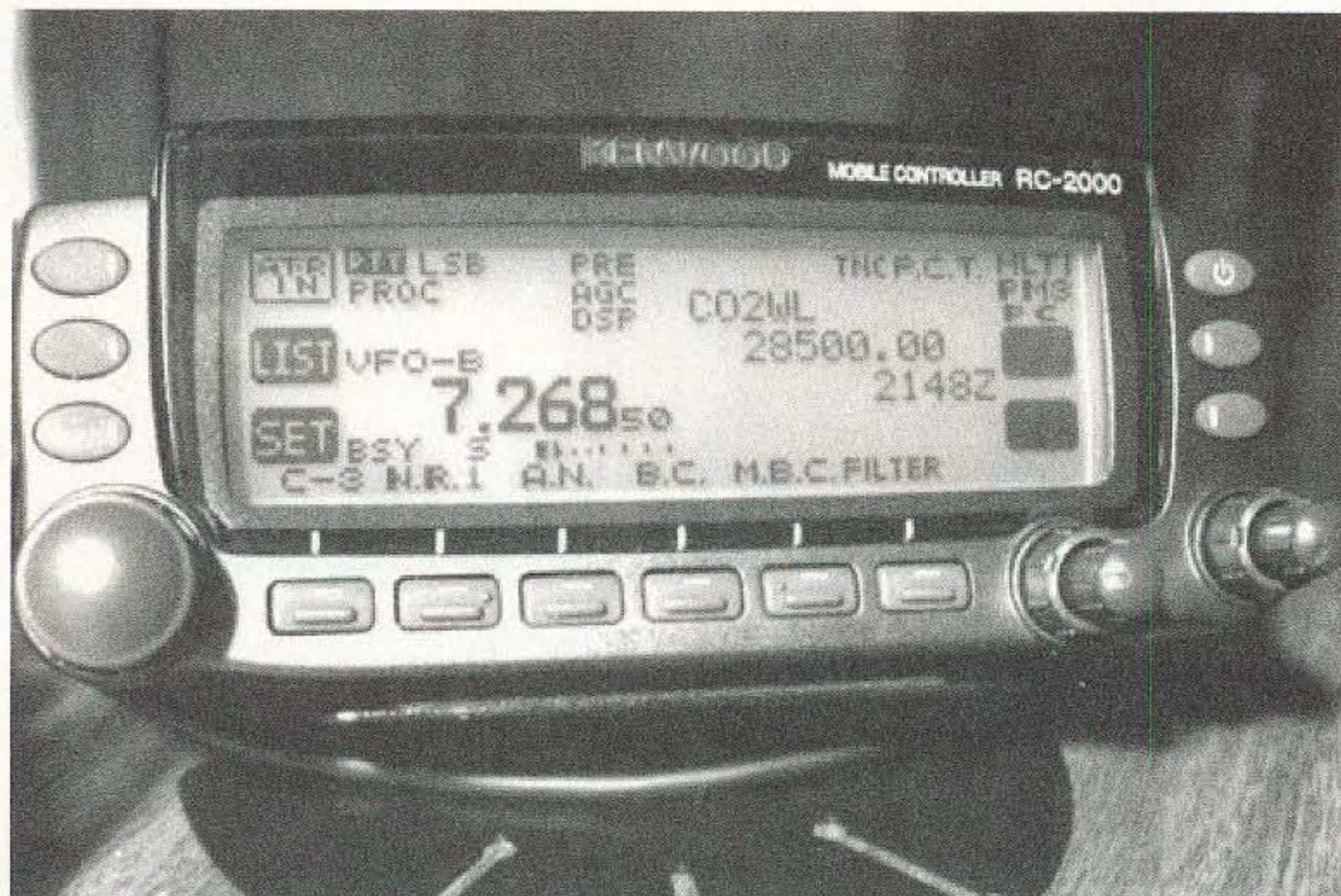
Photo D. Notice how the PCT DX spot information is displayed in an aesthetically pleasing cascaded fashion in the SUB window.
