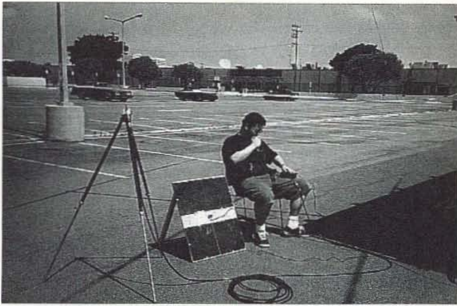
Photo C. Chris KF6RSV, operating the solar powered station. The vertical antenna was taped to a camera tripod, creating a stable mount as well as a ground plane for the antenna.
