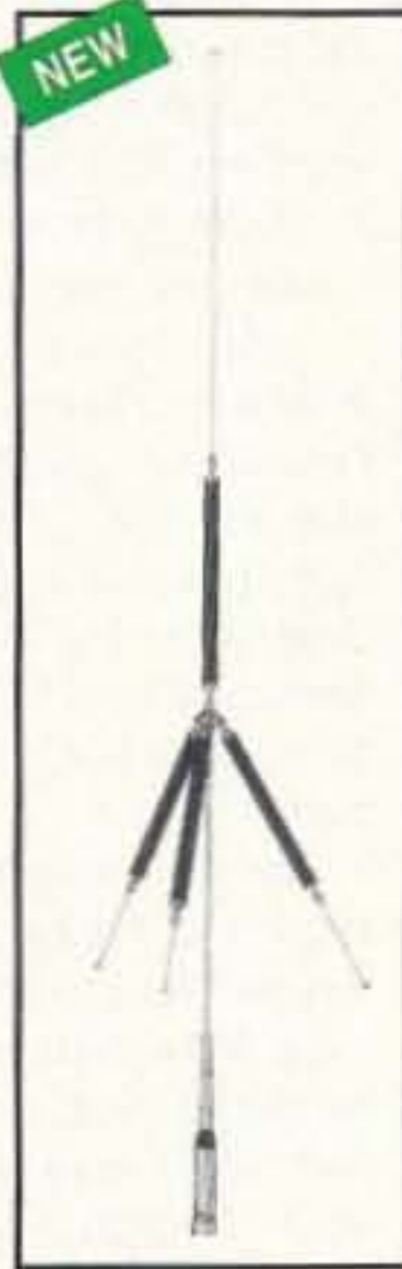
NEW HA4S Quad-Band HF Mobile 7, 14, 21, 24, 28MHz Wave: 1/4 wave VSWR: Less than 2:1 Weight: 1 lb. 14 ozs. Length: 4' 4" Connector: PL-259 Construction: Heavy Duty, w/fold-Over L-14HS: Optional 14MHz Coil
