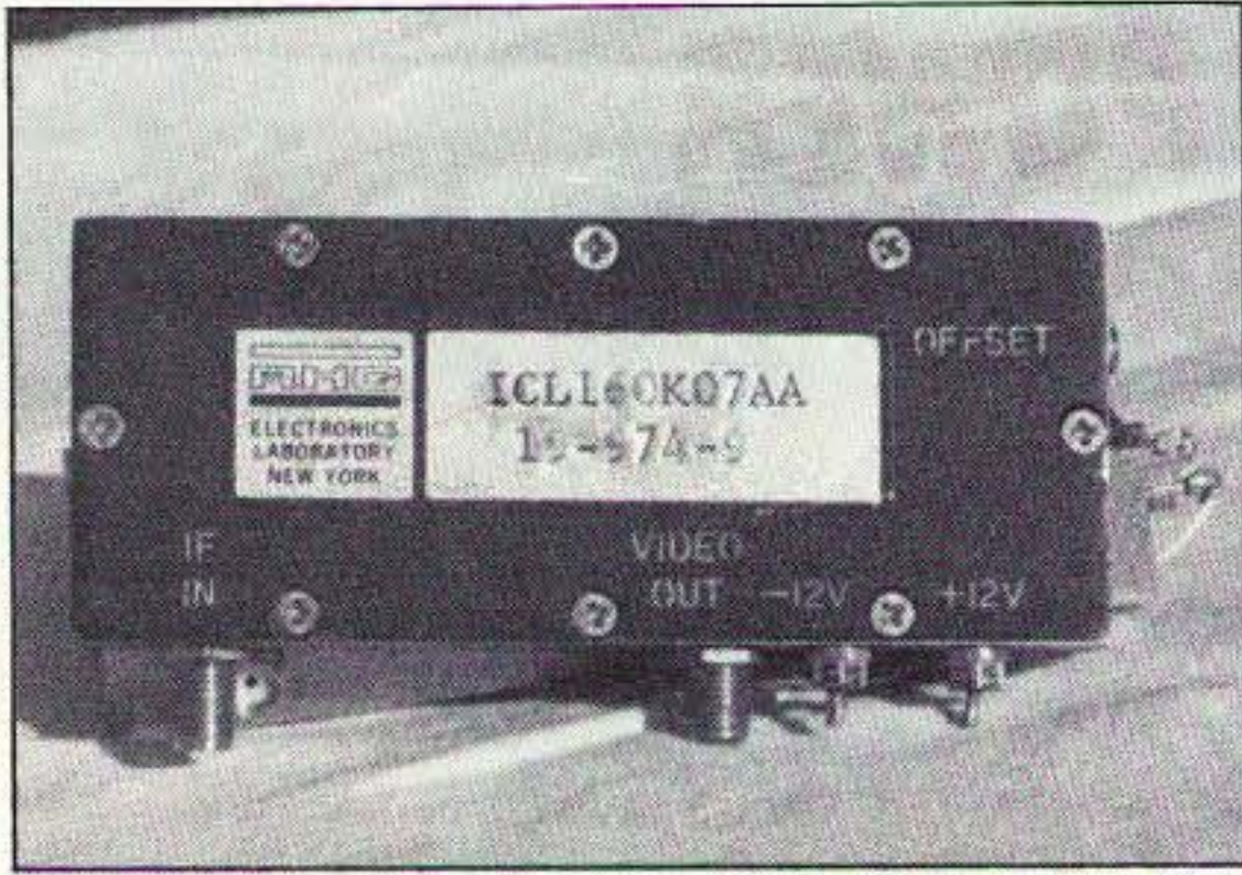
Photo B. New monolithic 160 MHz log amp 2-1/2" long. This one has 90 dB gain with 60 MHz dynamic range.
