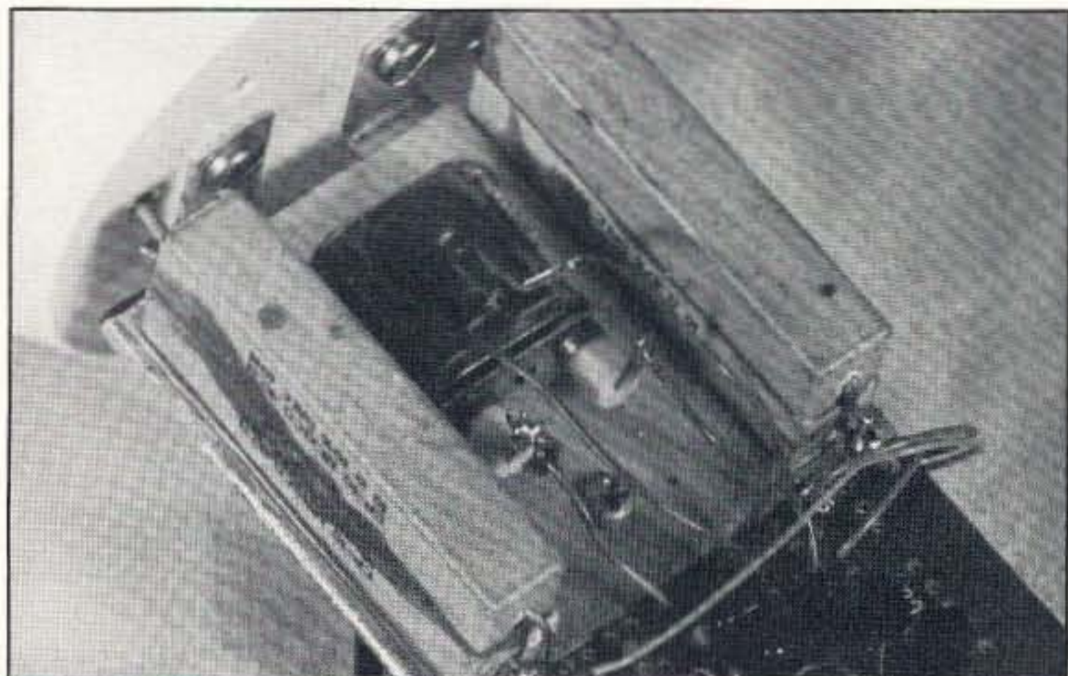
Photo C. Detail of the inner oven heater assembly. Note the heater resistors, crystal, and thermistor. The assembly is mounted to the top of the thermos bottle and to the end of the oscillator board prototype.
