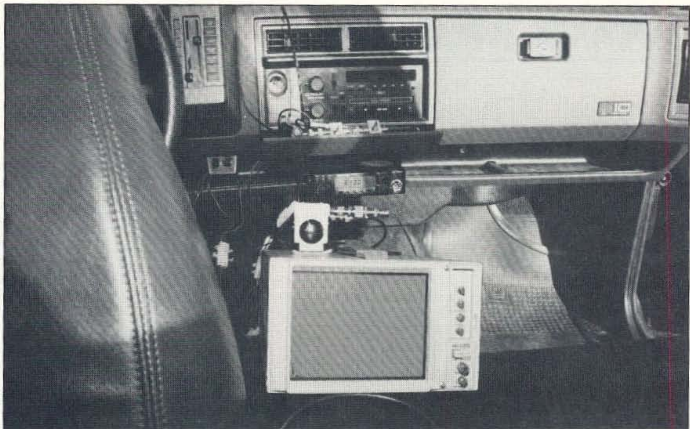
Photo G. Bill's storage oscilloscope readout sits astride the transmission hump and front seat, with RF attenuators mounted to the top.
