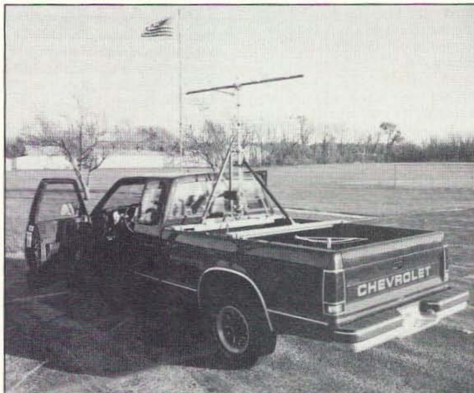
Photo A. His friends call it the "Foxcopter," but it never leaves the ground. Bill Rupp N0MKJ adapted a design of JaMi Smith KK6CU and built this motorized quad antenna for mobile RDF. (Photos by N0MKJ.)
