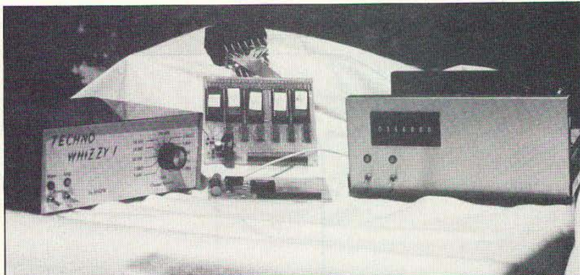
Photo D. The TW-1 DDS board surrounded by the new TW-1 and the original TW-1.
