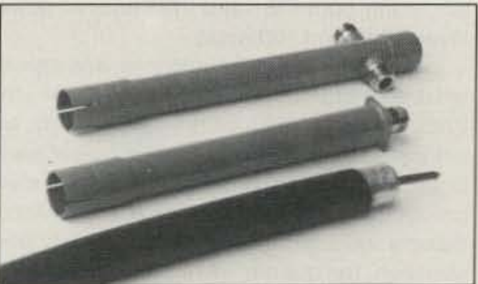
Photo C. 7/8" line prepared for installation of matching transformer and power divider.
