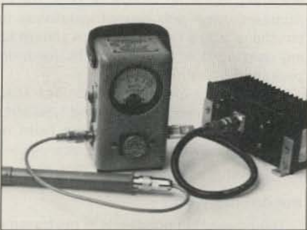
Photo B. 440 MHz Matching Transformer terminated in a 50 ohm dummy load.
