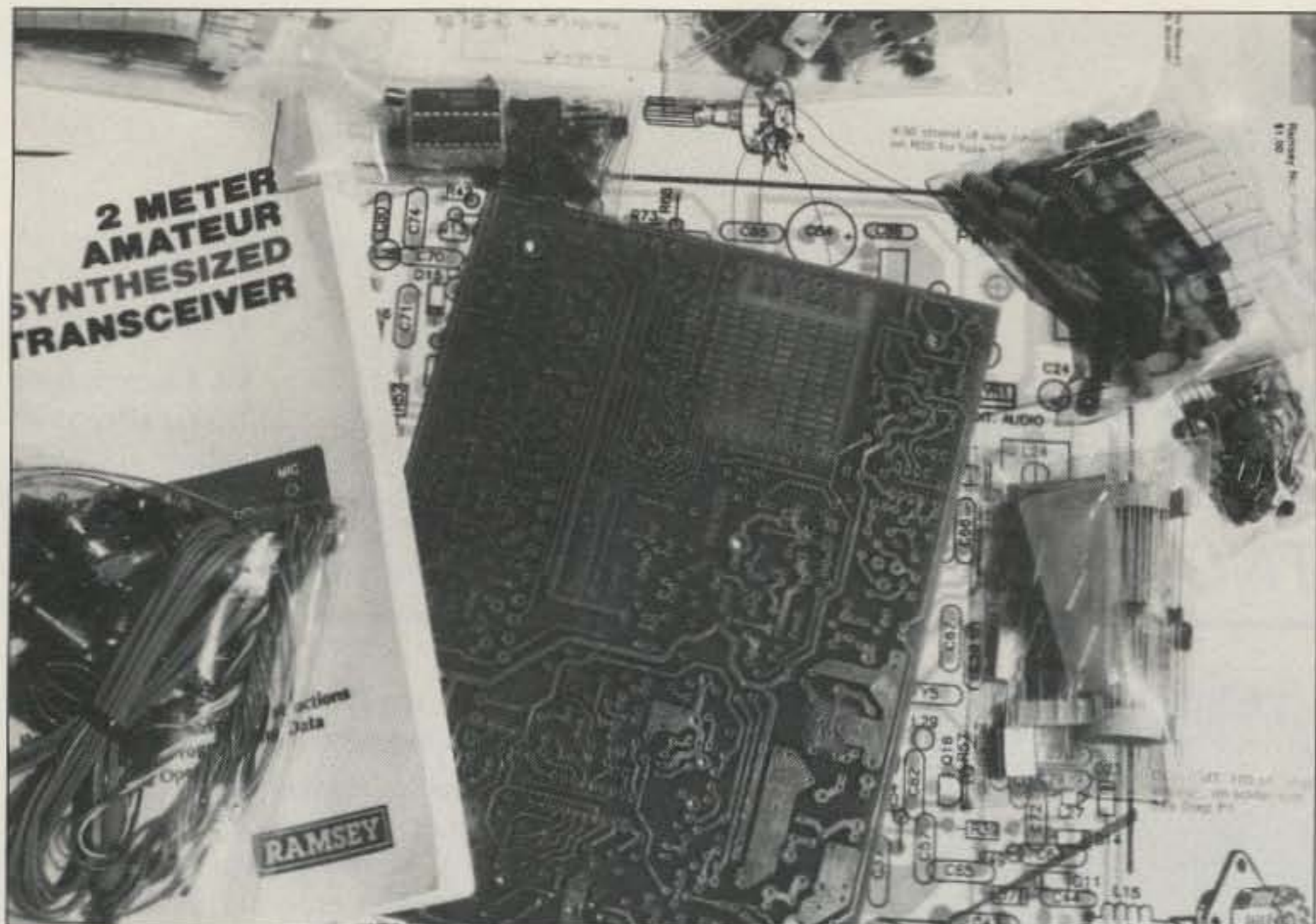
Photo C. The kit comes with a high-quality PC board, all components and excellent documentation.
