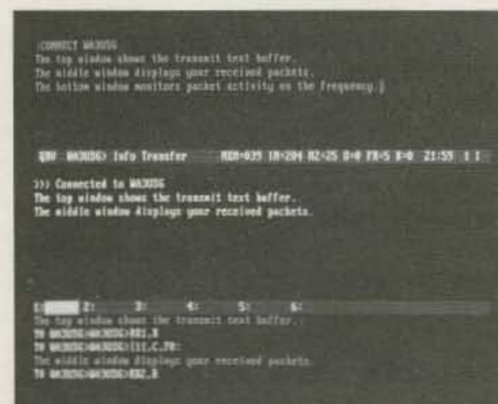
The terminal screen for the BayCom packet program. Three window area display transmitted packets, received packets and monitored packets.
