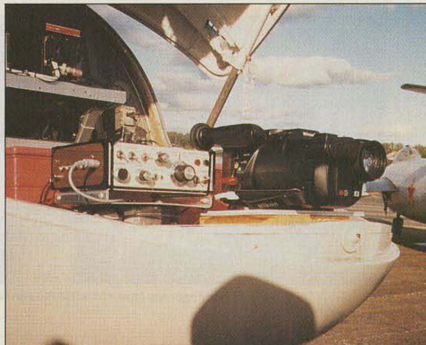
Photo D. Close-up view of the ATV installation. The P.C. Electronics TC70-1 was remotely controlled by touch-tone commands received by a small HT underneath the transmitter. An 8mm Ricoh camcorder not only provided the video signal for the ATV transmitter, but also recorded the flight on its video tape.
