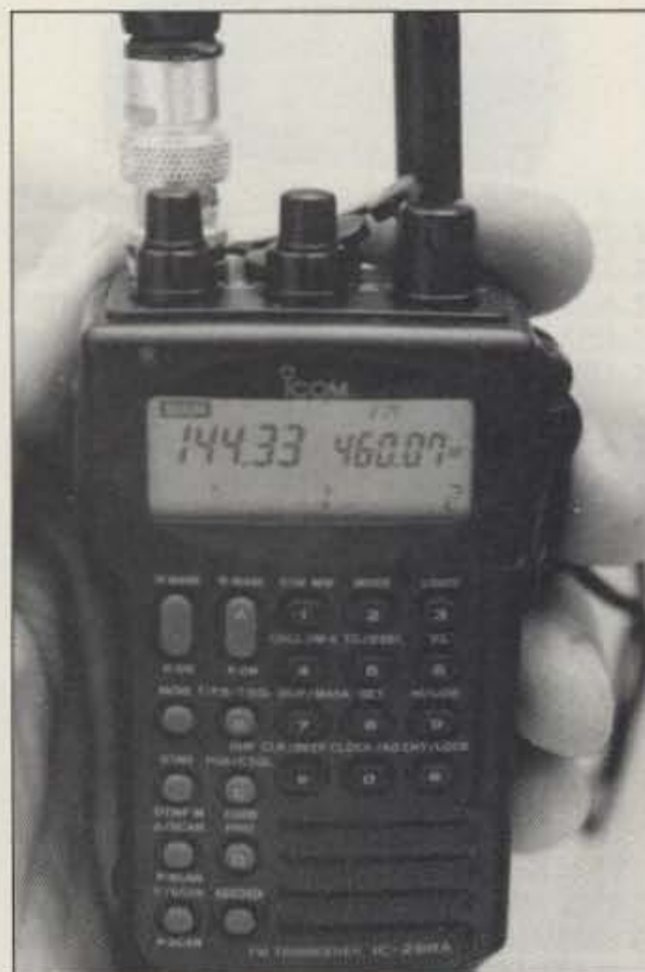
Photo A. The IC-2SRA, showing the 2 meter readout (left) and the scanner frequency readout (right).
