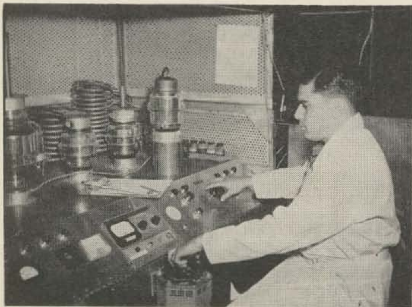
Leonard Espinosa operating Jennings Rig No. 3, a 20 KW linear amplifier with a 4 W 20,000 in the final.
