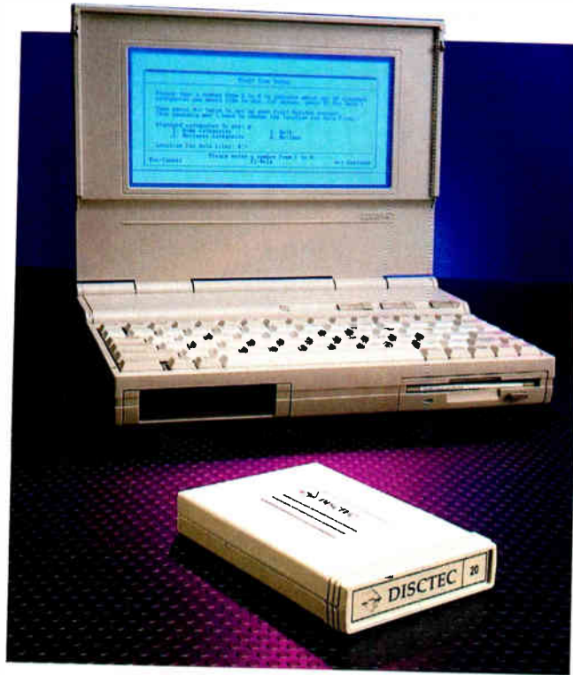
Disk Technologies' RHD 20 is a 20-MB removable hard disk drive that's fast and uses little power.
