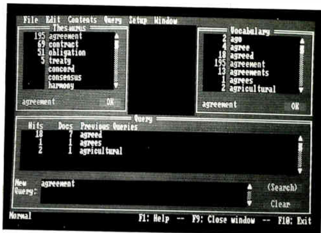
ZyIndex for Unix features two interactive tools that let you narrow a search for a word. The thesaurus box in the top left lists synonyms, while the box at right shows close approximations of the word. The screen at the bottom displays previous queries.
