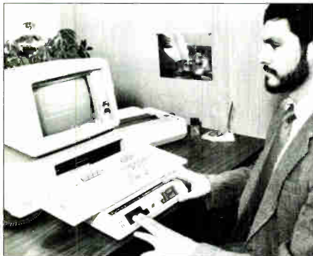
Photo 2: Blind people who use conventional computer keyboards can output what they have written on a braille printer, in speech, or on a braille display. Shown here is a user at a 40-column TeleSensory Navigator braille display unit consisting of a row of 40 8-dot cells. The top 6 dots display a standard braille symbol; the bottom 2 display character attributes and tell whether or not the cursor is on that symbol. Here the user reads the braille display with his right hand and manipulates the cursor with his left hand.
