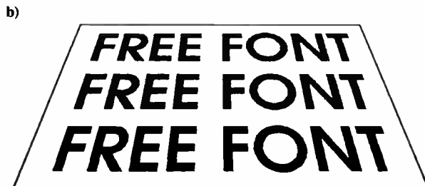
Figure 2: (a) This vertical pixel line remapping example prints in 70 seconds on a LaserWriter IINTX. By proc caching, or preconverting the image into 2 characters in a custom font, the repeat imaging time drops to 14 milliseconds, a 5000-to-1 speed improvement. (b) Star Wars-style lettering is one of the most popular uses for horizontal pixel line remapping. Each pixel line is shown somewhat shortened from the flat original. (See listing 1 for the method.) Since pixel remapping applies to any image, you do not need access to your font paths.
