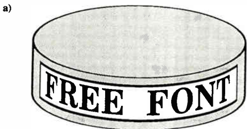
Figure 2: (a) This vertical pixel line remapping example prints in 70 seconds on a LaserWriter IINTX. By proc caching, or preconverting the image into 2 characters in a custom font, the repeat imaging time drops to 14 milliseconds, a 5000-to-1 speed improvement. (b) Star Wars-style lettering is one of the most popular uses for horizontal pixel line remapping. Each pixel line is shown somewhat shortened from the flat original. (See listing 1 for the method.) Since pixel remapping applies to any image, you do not need access to your font paths.
