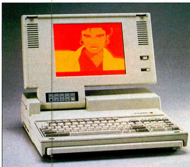
Fora's LP-386SX laptop features VGA graphics, floppy and hard disk drives, and a half-length expansion slot.
